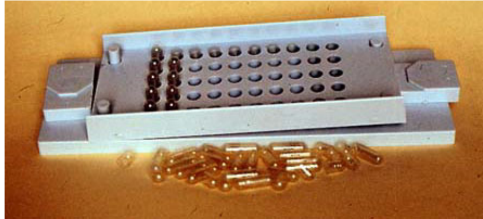
Figure 3.11: A small and cheap device for manually filling small quantities of hard gelatin capsules. With the top piece raised, as on the right, the pollen is brushed into the capsules. Once the top piece is lowered, as on the left side, the capsules can be closed.
