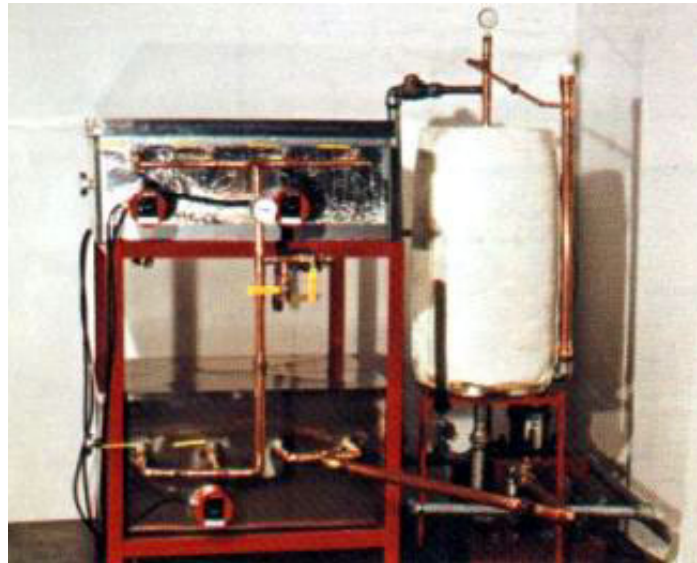
Figure 2.11 : Small to medium-scale vacuum drier for removing moisture from already extracted honey (courtesy of Dadant and Sons, Inc.).
