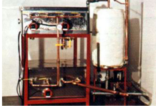
Figure 2.11 : Small to medium-scale vacuum drier for removing moisture from already extracted honey (courtesy of Dadant and Sons, Inc.).
