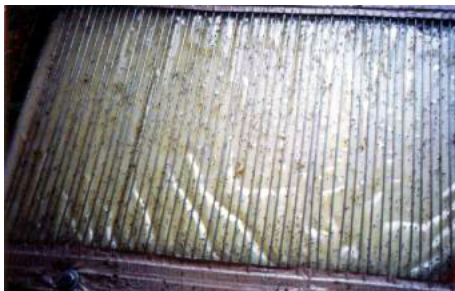
Figure 7.4 : Close-up of collecting device with stings. The steel wires are approximately 6 mm apart and suspended 1 to 3 mm above the
