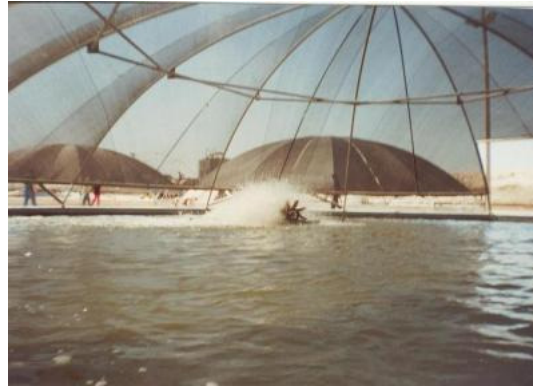
A paddle wheel aerator in action in an intensive fish farm i
