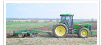
A modern John Deere 8110 Farm Tractor plowing a field using a chisel plow.
