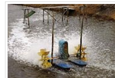
A one-horsepower paddlewheel aerator. The splashing may increase the evaporation rate of the water and thus increase the salinity of the pond.
