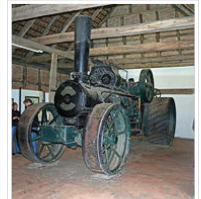
Ploughing engine Heumar , made by the Ottomayer company (Germany), used in pairs with a balance plough. Built 1929, 220 PS, 21 tons.
