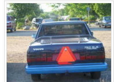
An "A tractor" based on Volvo 760. Notice the slow vehicle triangle and the longer boot.
