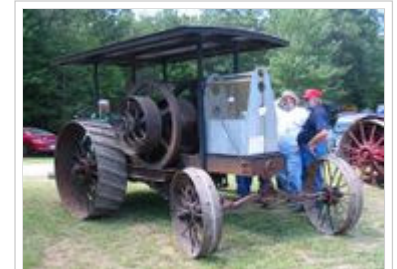
A 1920 International Harvester tractor, showing features inherited from earlier steam tractor designs.
