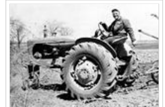
The classic Row Crop tractor (an Allis-Chalmers WD). Note the absence of any rollover protection system.
