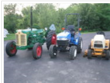
In the middle is a 24 hp (18 kW) diesel CUT illustrating the size difference between a small farm tractor and a garden tractor
