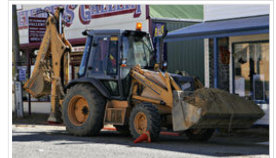
A common backhoe-loader. The backhoe is on the left, the bucket/blade on the right.
