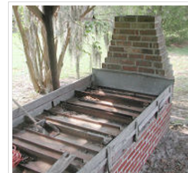
Evaporator with baffled pan and foam dipper for making ribbon cane syrup. Three Rivers Historical Society Museum at Browntown, South Carolina
