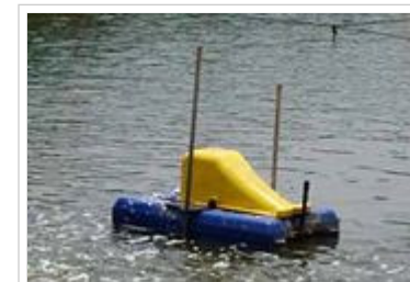
The intake of a two-horsepower "Turbo aerator", which paddles one metre below the water surface. To avoid stirring up pond sediments, the water depth should be at least 1.5 m.
