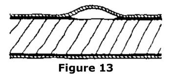
Glue bulges are rolling glue piles under the veneer face.
