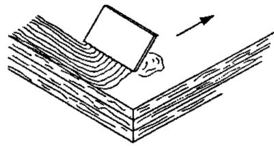
Figure 12 - Putting on glue with a putty knife
