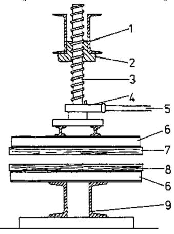
Figure 2 - Press (cut-away model)
