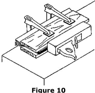
After this job the veneer faces are placed together separately. The joint density can be checked by pressing the two veneer sheets together at the joint edges. Now the joint should be unvisible.
