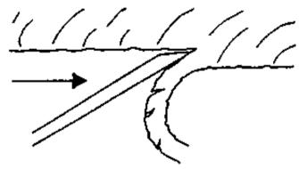
Figure 8 - Principle of veneer production
