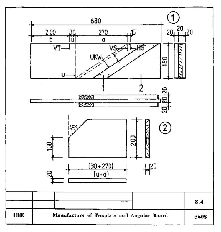
Manufacture of Template and Angular Board
