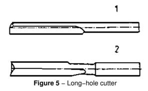
1 with one cutting notch, 2 with two cutting notches
