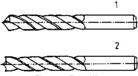
Figure 4 - Twist driller
