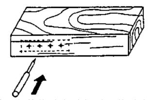
Figure 9 – Marking the long hole and punching the bores
