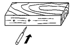
Figure 7 – Marking and punching of the bore centres
