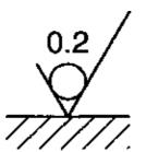
Roughness value must be obtained without removal of material.
