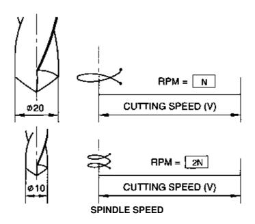
The RPM of the drill depends on the <u>cutting speed</u> and <u>diameter</u> of the drill.
