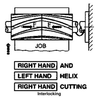
Cylindrical milling cutters with helical teeth directed against each other have the advantage that the axial pressure is partially compensated
