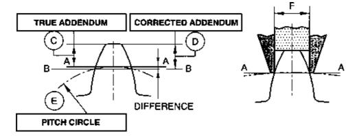
After calculating the corrected addendum and chordal thickness the gear tooth vernier is set to the calculated value and the gear tooth checked.
