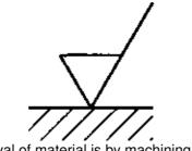
Removal of material is by machining only.
