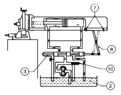
At the end of the forward stroke the reversing dog (7) hits against the reversing lever (8) causing the reversing valves (9) to alter their position within the valve chamber (3). Oil under high pressure is now made to flow to the left side of the piston causing the ram to move back (return stroke).
