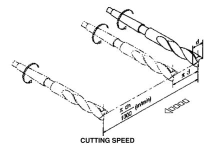
The cutting speed for drilling is the speed of the periphery of the cutting edge in m/min.
