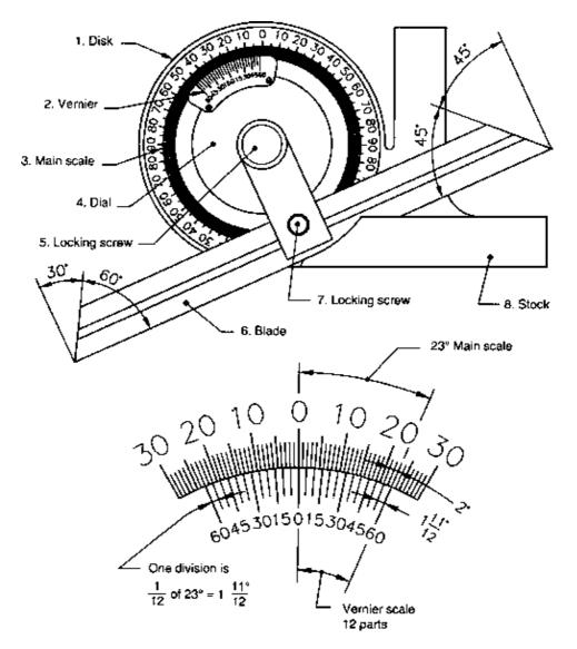
The full circumference of the disk is graduated into 360 equal parts.
