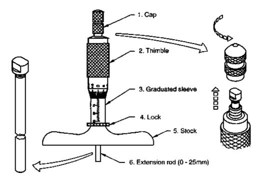
The extension rod face flushes with the stock when zero of thimble coincides with the zero of sleeve
