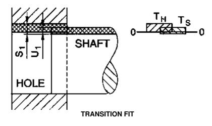
$S_1 = Maximum Clearance$  $U_1 = Maximum Interference$
