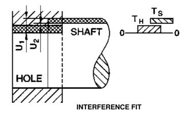
$U_1 = Maximum Interference$  $U_2 = Minimum Interference$
