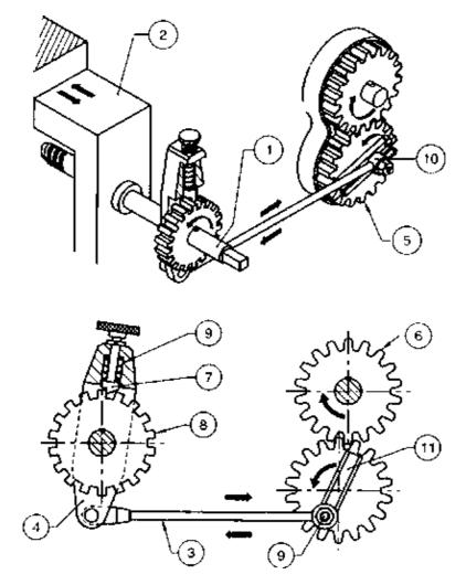
The cross feed screw rod (1) is connected with the table (2). The connecting rod (3) connects the Pawl arm (4) and the crank wheel (5).
