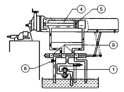
The oil under high pressure due to gear pump (1) is pumped from the reservoir (2). This oil passes through the valve chamber (3) to the right side of the cylinder (4) exerting pressure on the piston (5). This causes the ram to move in forward direction. (Forward stroke)
