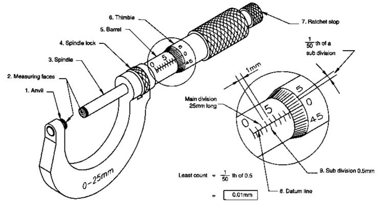
The range of the Micrometer is 0 – 25 mm.
