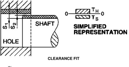
$S_1 = Maximum Clearance$  $S_2 = Minimum Clearance$
