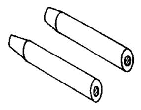
2 x round material made of silver steel (1.1 to 1.25 % of carbon)
