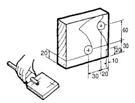
Use a brace and a 20mm bit to drill out the two holes. The shape of the handle can then be drawn in.
