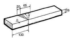
Set a marking gauge to 26mm and gauge the width of the throat on each piece, top and bottom.
