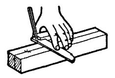
Gauge each piece to a thickness of 38mm. The waste will be planed off after the stock has been glued together.
