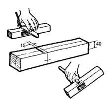
Gauge a line on each side of the stock to meet the pencil lines, 40mm from the sole. This marks the centre of the holes for the crossbar.
