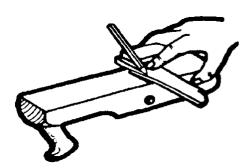
Square a line on the sole, 2mm from the front of the mouth. Use a wide chisel to pare straight down into the front of the throat. Repeat this process until there is a gap of about 3mm or 4mm between the cutting edge and the front of the mouth.
