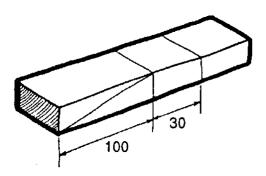
Clamp the wedge vertically in the vice and use a ripsaw to cut the angle. Plane the sawn face by clamping it in a vice horizontally, with a small piece of timber to support the thin end.
