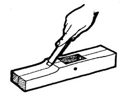
down to the gauge line, on both sides.
