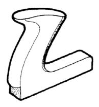
Finally, carve the handle smooth and round. The chamfers should help to make the curves even. A fine half-round file and some sandpaper will help to finish the handle well. When the handle is finished it should look like this.
