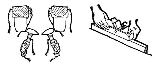
Look along the bottom of the plane to make sure the cutting edge is parallel to the sole. If one corner is too high then tap the opposite side of the blade. Repeat these actions until the plane cuts a fine, even shaving.
