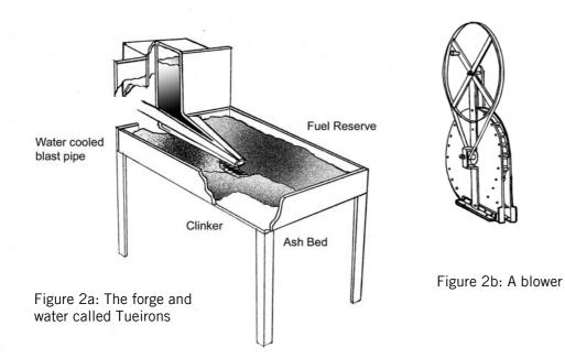
The traditional bellow and some crank fans require manual input; another option is an electric fan where available.
