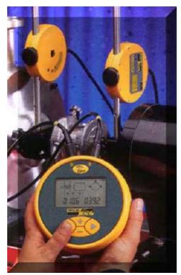
LASER BASED SHAFT ALIGNMENT TOOL
