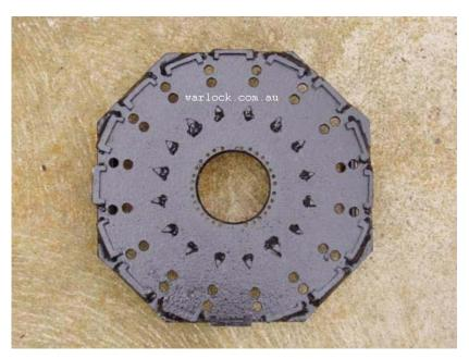
Figure 2. Front half of generator rotor
