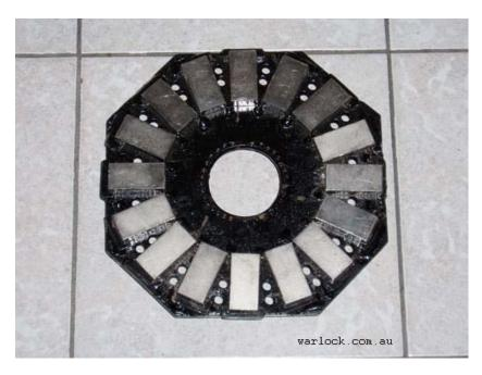
Figure 4. Front half of generator rotor with magnets attached
