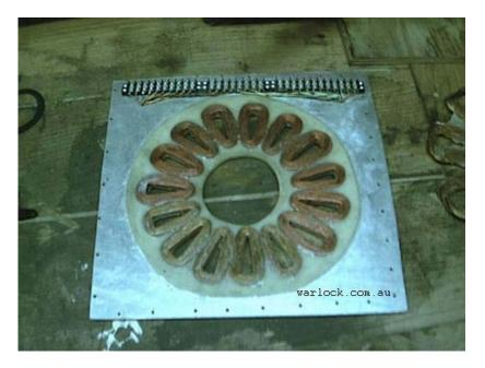
Figure 3. Generator stator
