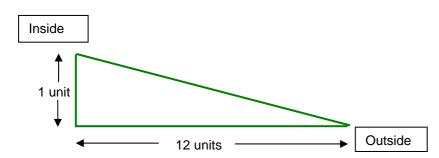
Construction of a ramp should consist of minimum 4'- 0" width (wide). It should consist of thick brick kerbs on both sides, preferably 9" in thickness (in cement and sand). The rubble foundation as shown in figure 1 should be constructed as 12" x 12" in depth using cement and sand 1:5.
