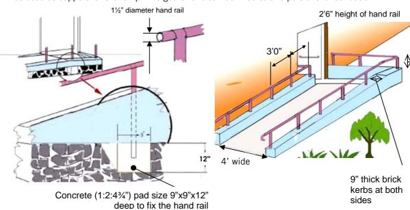
Figure 4: Placing handrails in the foundation
