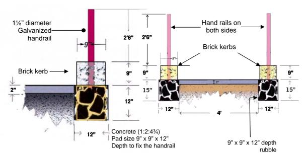
Figure 2: Fixing handrails
