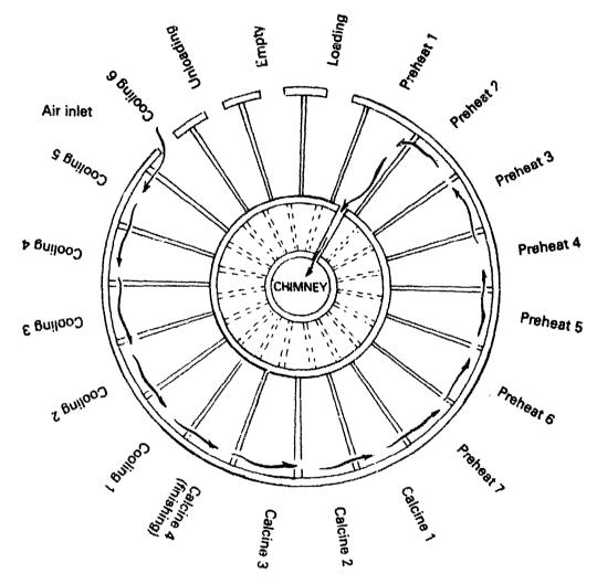
Diagram of chambers in a ring kiln.
