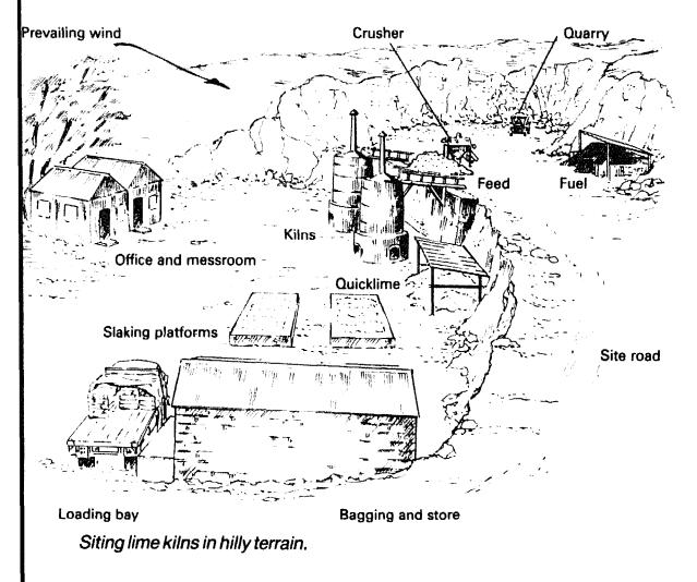
If the kiln is at the quarry it should be reasonably close to the workface. When the feed material is delivered to the site by lorry, a well-made access road should be taken right up to the top of the site so that lorries can be unloaded immediately by the kilns.
