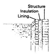
Batch kiln — insulation close to the inner face.
