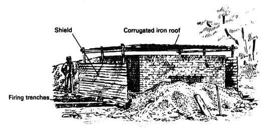
A very simple flare kiln for a road construction project in Ghana (Transport and Road Research Laboratory).
