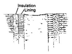
Shaft kiln — more masonry within the insulation.
