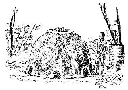
A heap covered with clay daub.
