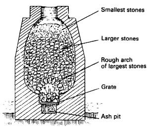
Cross-section of a loaded pot kiln.
