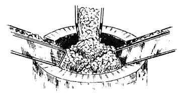
Reducing separation by charging through three chutes.
