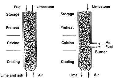
Vertical sections through mixed feed and separately fired vertical shaft kilns.
