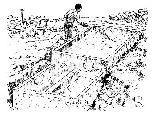
A hand slaking tank with two settlement tanks.
