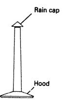
A galvanized iron chimney for a KVIC shaft kiln.
