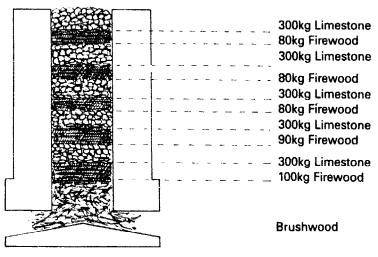
The initial charge for mixed feed continuous firing.
