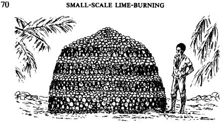
An uncovered heap with alternative layers of wood and limestone.
