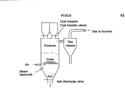
Scheme of gas producer using coal.
