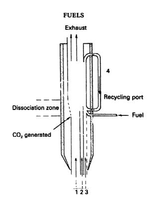
Diagram of gas flows through a kiln.
