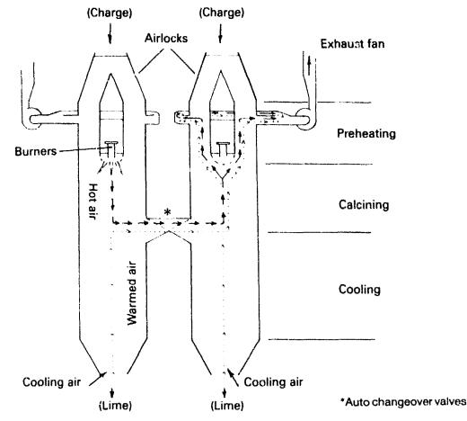
Cross-section of a parallel flow shaft kiln.
