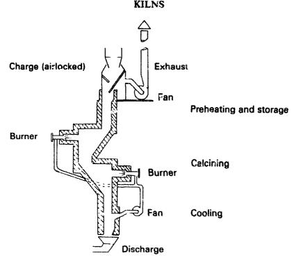
Double inclined vertical kiln.
