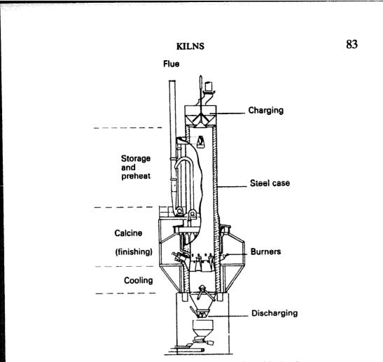
A separately fired shaft kiln designed by Wests Pyro Limited.
