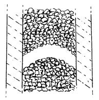
'Arching' of the charge in a shaft kiln.
