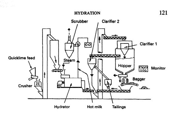
Flow plan of mechanical hydration plant by Fletcher and Stewart Ltd.
