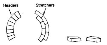
Radial headers and curved stretchers are special bricks for circular structures. Refractory linings are available in these shapes.
