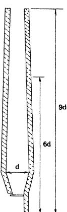
The height of a shaft kiln should be at least six times the diameter and preferably nine times.
