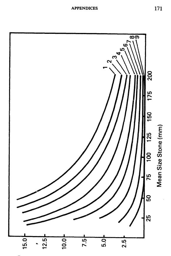
Pressure drop through kiln  $\triangle$  p (mm W.g.)
