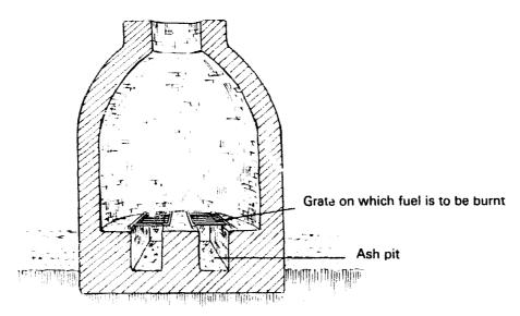
Cross-section of a flare kiln with two grates.
