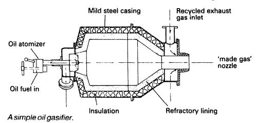
recycled for flame attenuation and for temperature contol in the kiln. Appendix 12 includes some of the properties of the gas made during trials with a 3500secs heavy residual fuel oil. Other trials were run using lighter oils and the results were very similar.
