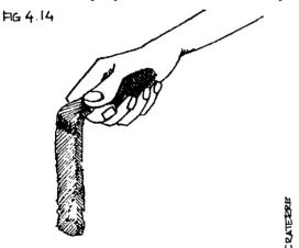
This is a simple way of testing the soil on site.
