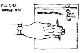
Quickly take the sample, put it in an airtight container and weigh it. Subtract the weight of the container and record the result. Dry the sample and weigh it again. The plastic limit is the weight of the water (the difference between the wet and dry weight) divided by the dry sample weight, and the result multiplied by 100 to get a percentage. If the results from each half sample differ by more than 5%, do the test again.
