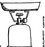
Some of the tests which follow require the soil to be dried before or after testing. This can be done in an oven, at a constant temperature of 105 - 110°C, over a period of 8 hours or more, or in a pan over a gas or paraffin pressure-stove. Stir the soil around whilst it is drying, which takes an hour or more depending on its dampness.
