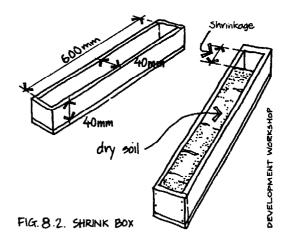
Push all the soil, including separated lumps, tightly up to one end of the box. Measure the gap created by the shrinkage in the soil. The results can be interpreted (\*1) as follows:
