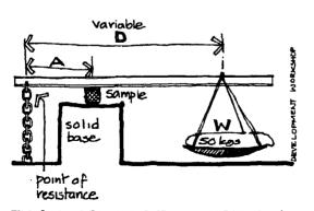
FIG 5.1. APPARATUS FOR COMPRESSION
