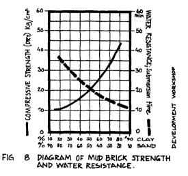
With a high clay content soil, one can add sand, if this is conveniently available. Straw can be added to reduce the risk of cracking when drying, to improve the tensile strength, and to lower the weight of the block. As a guide, allow 5kgs straw per  $1m^3$  soil when the sand content is less than 50%, and as much as 15kgs per  $1m^3$  if the sand content is as low as 30%.
