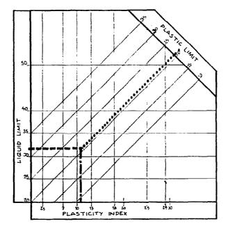
SOIL EXAMPLE LIQUID LIMIT - 32 PLASTIC LIMIT = 21 PLASTICITY INDEX = 11
