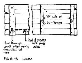
The ties, of whichever type, connect with the vertical posts. The spacing of ties and vertical posts along the length of the form depends upon the thickness of the form. Using planks 30 - 35mm thick, the posts can be spaced at 0.65 - 0.70m centres, further apart with thicker planks, and closer together with thinner. Plywood may need additional horizontal bracing.
