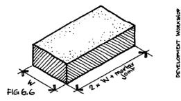
Bricks or blocks can be square or rectangular. When square they should ideally be the same width as the to simplify bonding without wall. much cutting of bricks. requiring Small square bricks can be used in combination with rectangular bricks of half the width, although one then careful calculation for the needs number of each type.
