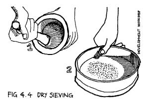
From these two tests - sedimentation and dry sieving - one has established the proportions of each particle group. A typical soil suitable for use in mud bricks could have the following proportions: sand 40-75%; silt 10-30%; clay 15-30%.
