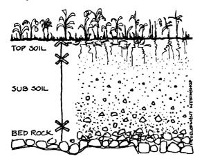
Although the depth of soil varies, in general if a vertical cut is made in the soil it will show that the soil is made up of layers, varying in texture, colour and depth. There may many different layers, but a be typical profile of a soil can be divided into three parts: topsoil, containing large quantities of organic matter; subsoil, containing little or no organic matter; and bedrock, which may or may not be broken down into lumps.
