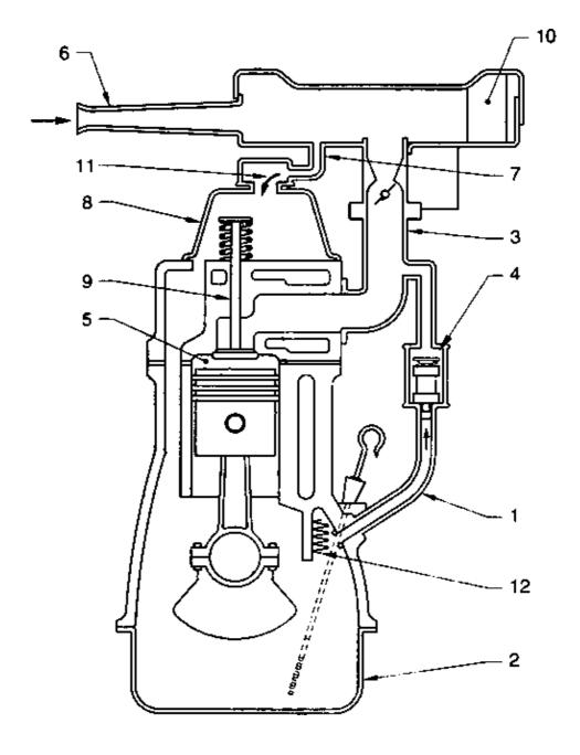
In IC engines, products of combustion leak past the rings into the crankcase. These products are to be removed to reduce oil contamination, dilution, corrosion and other undesirable chemical effects. For removal of these products positive crankcase ventilation is used in engines.
