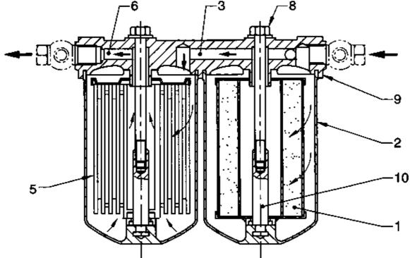
In a Diesel Engine a number of fuel filters are used to clean the fuel free of contaminants to enable the fuel to pass through clearances of very highly precision finished parts like Elements and Nozzles.
