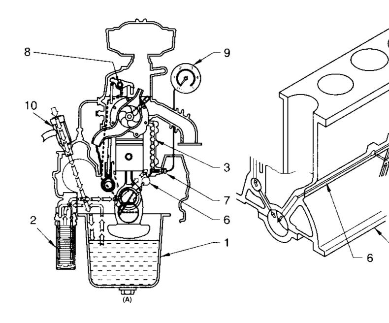
Diesel Engine Lubrication oil filter (full flow)
