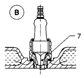
In this plug, the heat travel path/Insulator base (7) is shorter. Hence plug is cooled quicker by cooling water in the jacket (2). It works comparatively cooler. Hence it is called as "Cold Plug" (B).
