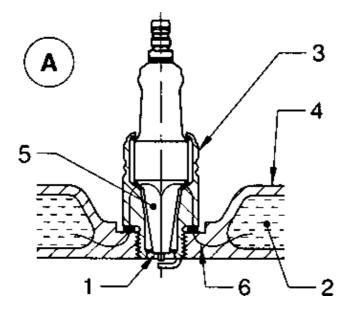
The travel of heat in a Hot plug (A) is shown. The heat travels from Insulator nose (1) and reaches the cooling water (2) through shell (3) and cylinder head (2). The Insulator Base (5) is long and so heat travel path (6) is also long. Hence it is called as Hot Plug (A). The Insulator Nose (1) is the hottest part of a plug, which determines the "Heat Range". The Nose of Insulator Projects into combustion chamber. The Hot Plug vaporises carbon deposits quickly.
