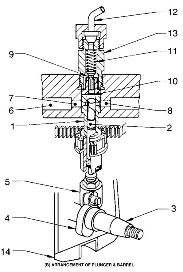
Working of F.I.Pump (Fig B)
