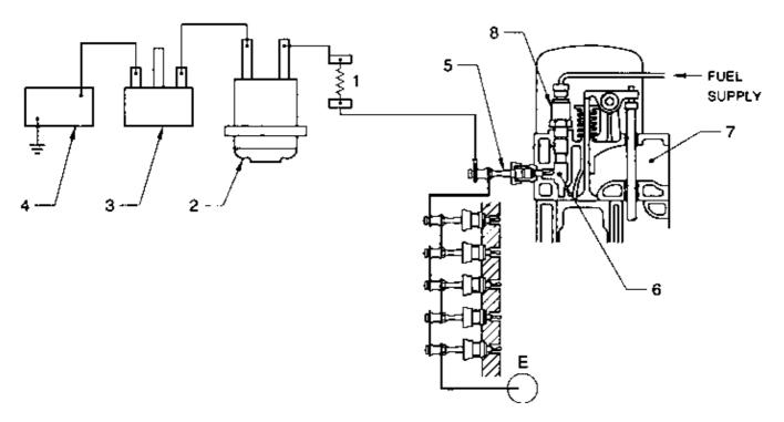
In this system Glow Plug resistor (1) and pre-heating monitor (2) are connected in series. The line resistor (1) and the preheating monitor (2) provide for the over all electrical resistance of the pre-heating system to match with battery voltage.
