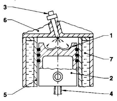
This combustion chamber (1) is provided on the top of piston (Crown) (2) in the form of cup shaped recess called "TORRIDAL". A swirling motion with squish is provided by the air when it passes into the Torridal chamber. The mixing of fuel and air is good and quick.
