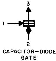
CAPACITOR-DIODE GATE, POSITIVE OR NEGATIVE INDICATED BY POLARITY OF THE INPUTS.
