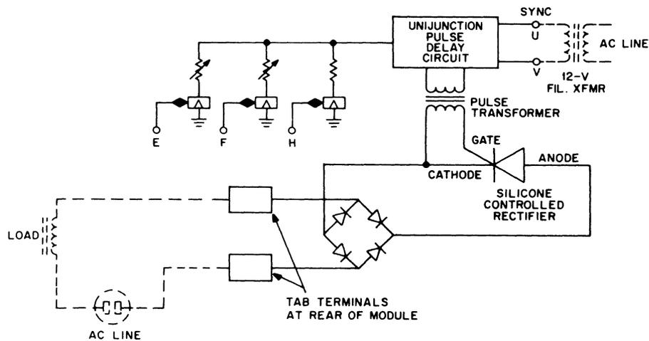
Figure 2-3 Symbolized Schematic of G850 SCR Motor Driver
