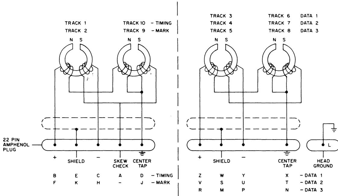
Figure 2-2 Head Connections
