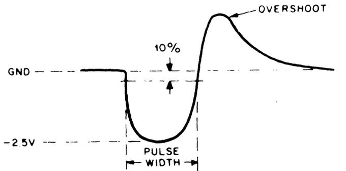
Figure 5-3 FLIP CHIP B-Series Pulse
