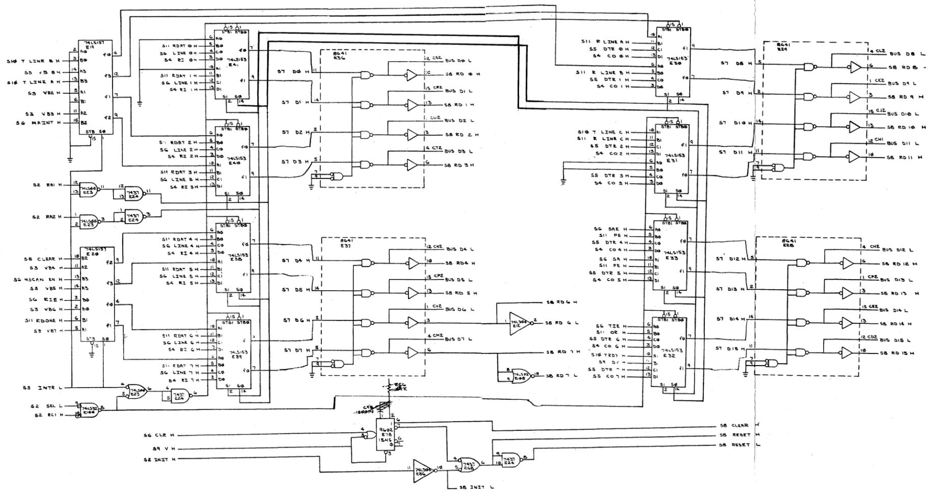
Figure 4-9 Unibus Data Flow
