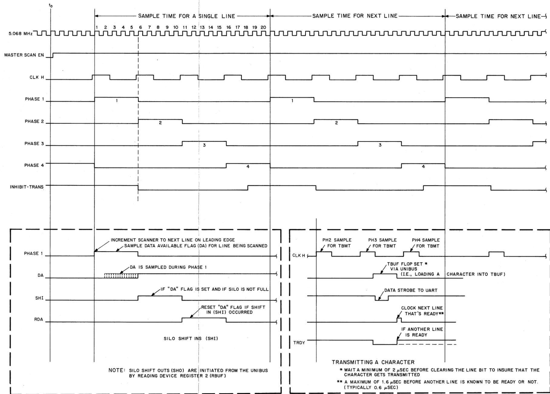
Figure 4-12 DZ11-A Scanner Timing
