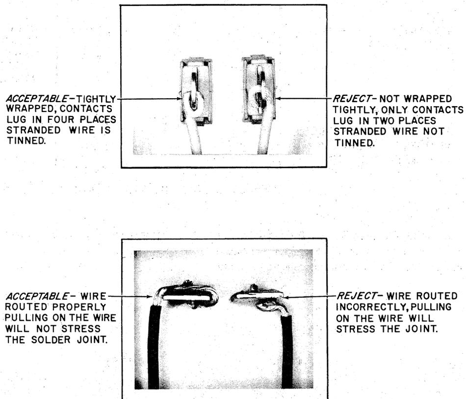
Figure 5-15 Example of Wire Joint Before Soldering
