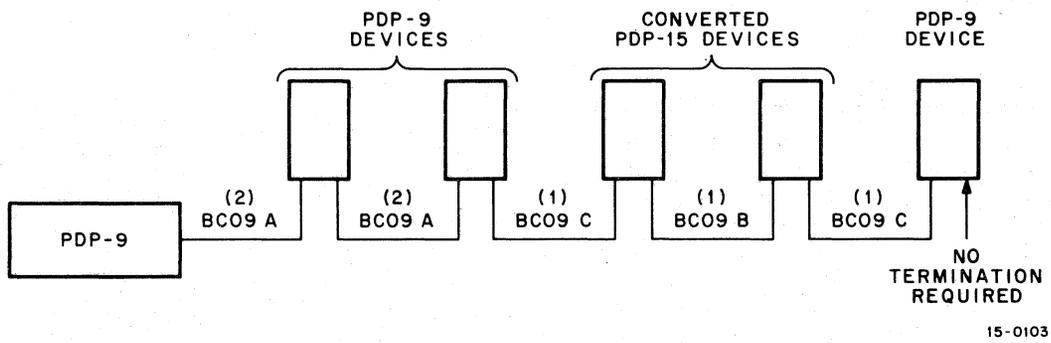
Figure 6-9 Cabling Converted PDP-15 Devices to the PDP-9 I/O Bus
