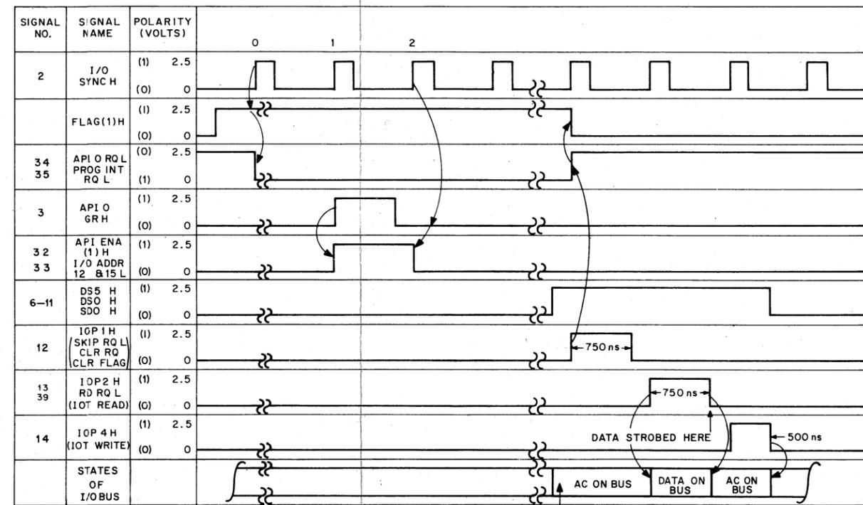
Figure 4-4 Timing Diagram of the CPU Device with API
