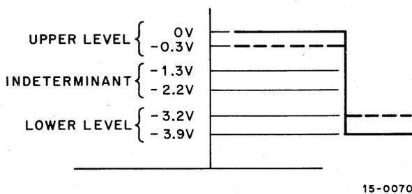
Figure 2-1 Voltage Spectrum of Negative Logic Systems
