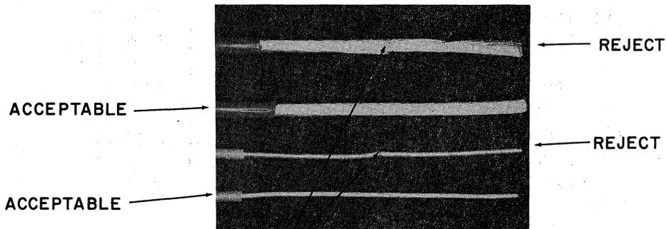
CONDUCTOR IS NICKED BY AN IMPROPERLY ADJUSTED WIRE STRIPPER.
