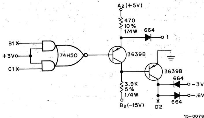
Figure 2-15 M632 Schematic
