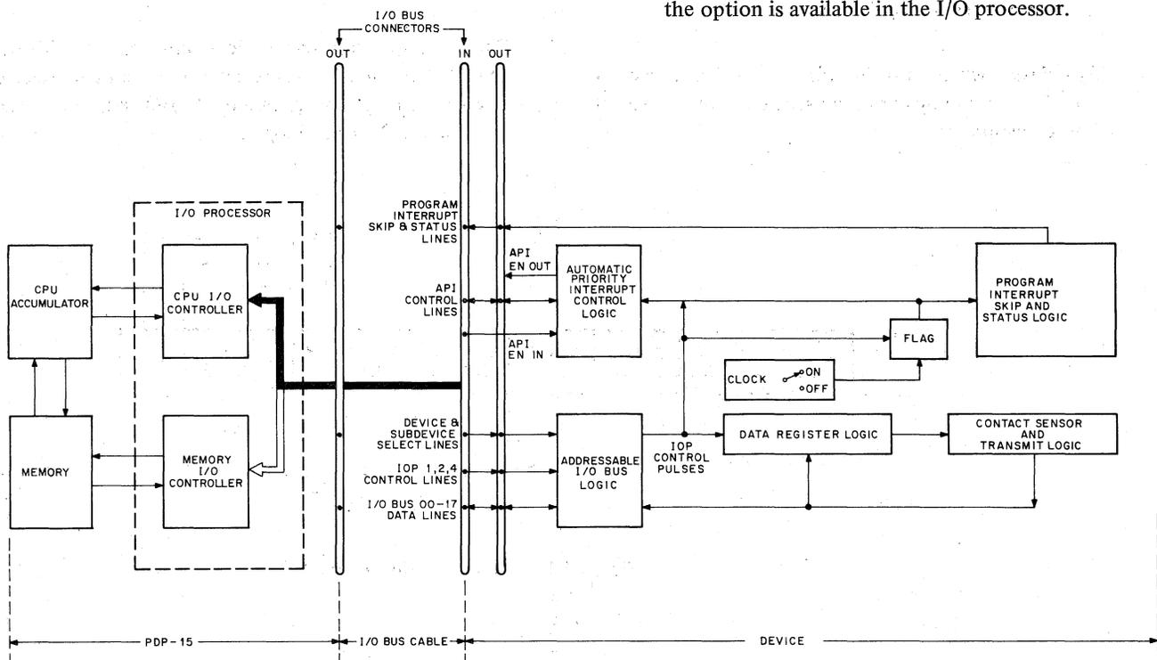
Figure 4-2 Block Diagram of CPU Device with API
