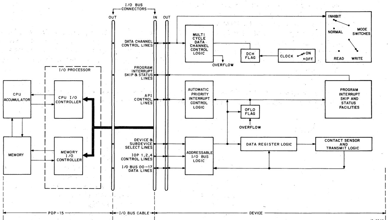
Figure 4-5 Block Diagram for Multicycle Data Channel Device
