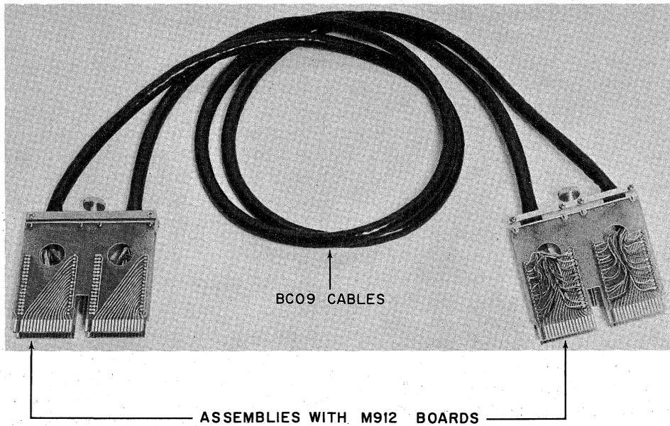
Figure 6-5 BC09B Cable Assembly
