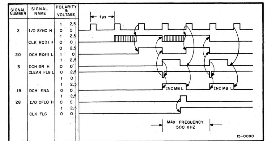
Figure 4-10 Timing Diagram for Increment Memory Devices
