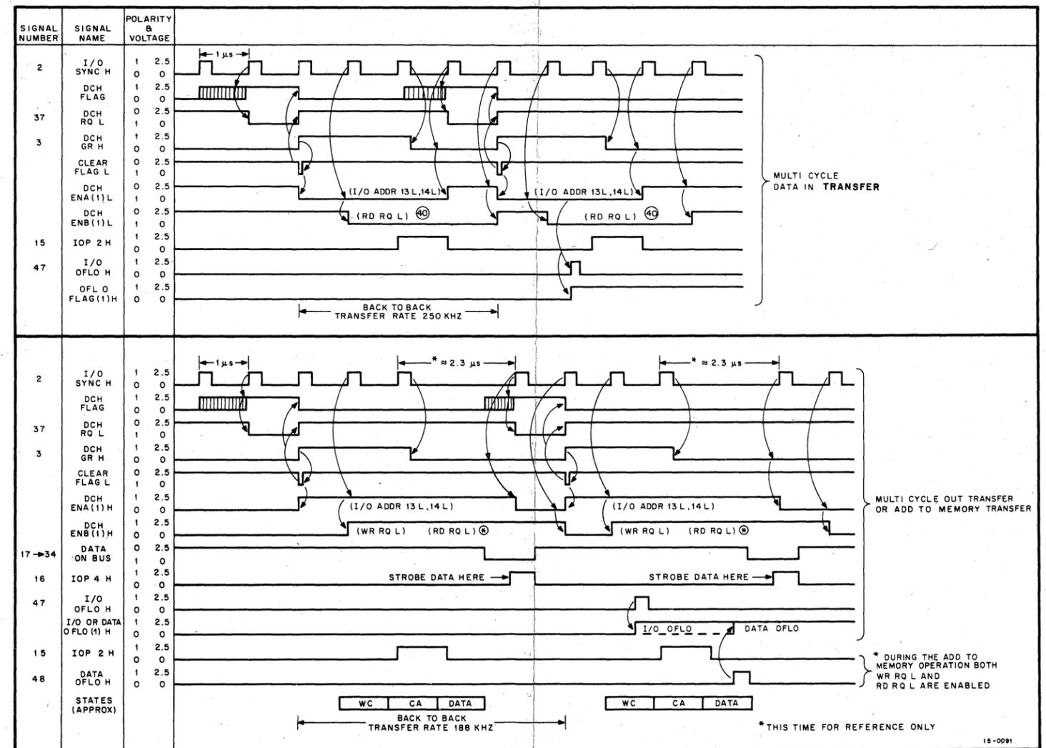
Figure 4-7 Multi-Cycle Data Channel Timing
