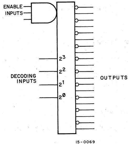
Figure 1-14 Binary to Decimal Decoder
