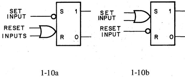
Figure 1-10 R-S Flip-Flop
