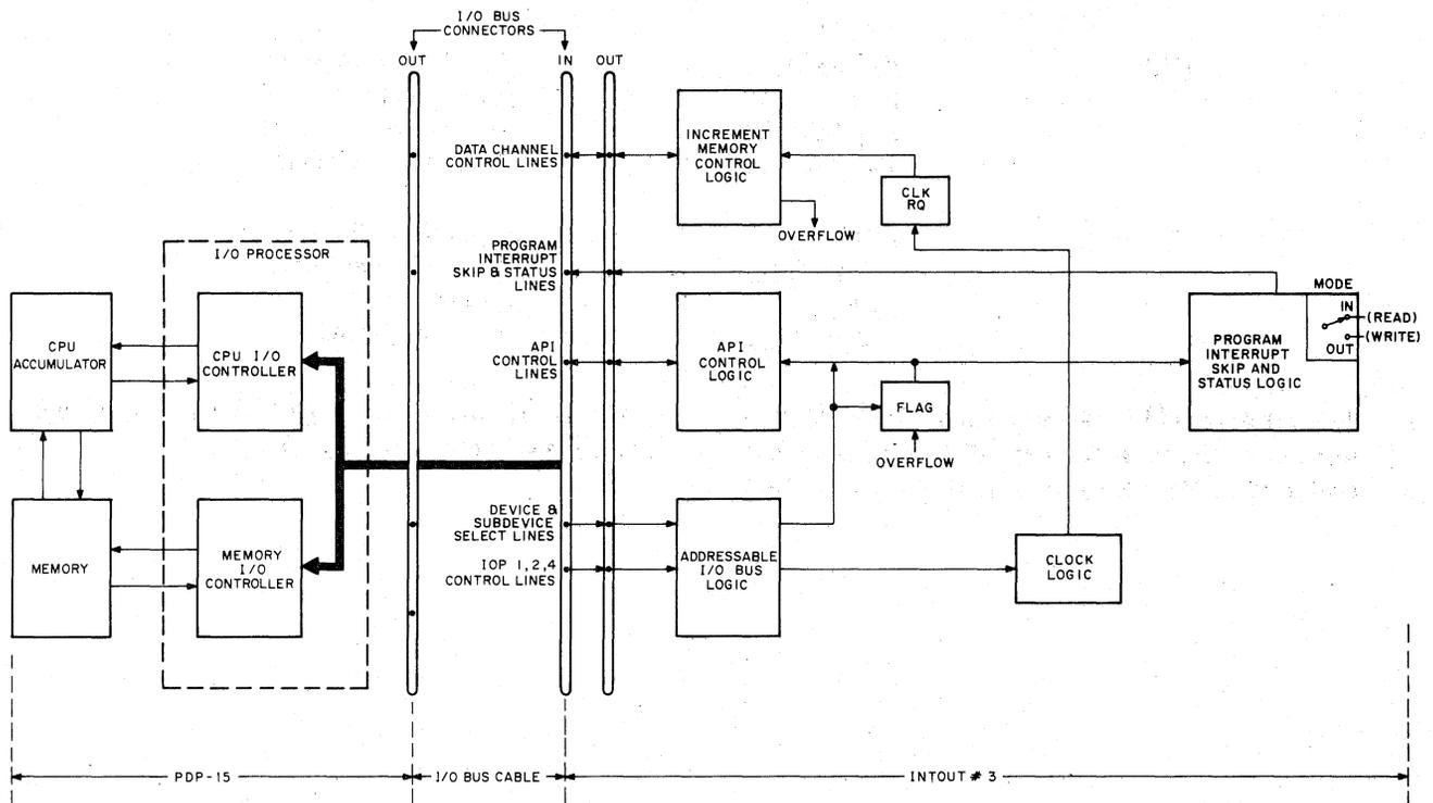
Figure 4-8 Block Diagram for Increment Memory
