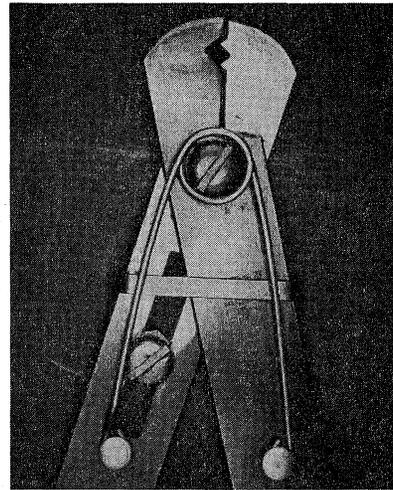
Figure 5-7 Adjustable Wire Stripper (Use With Caution)
