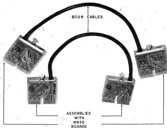
Figure 6-2 BC09A Cable Assembly
