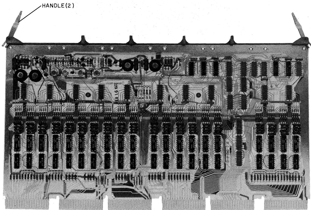
Figure 3-2 Component Side of Drive Module G231
