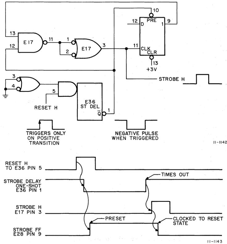
Figure 3-29 Strobe Generating Circuit and Timing Diagram
