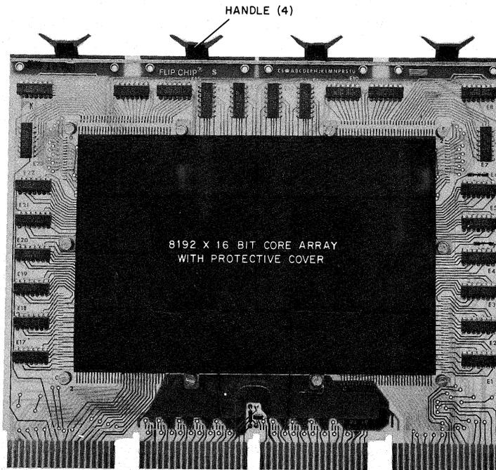
Figure 3-3 Component Side of 8K Stack Module H214
