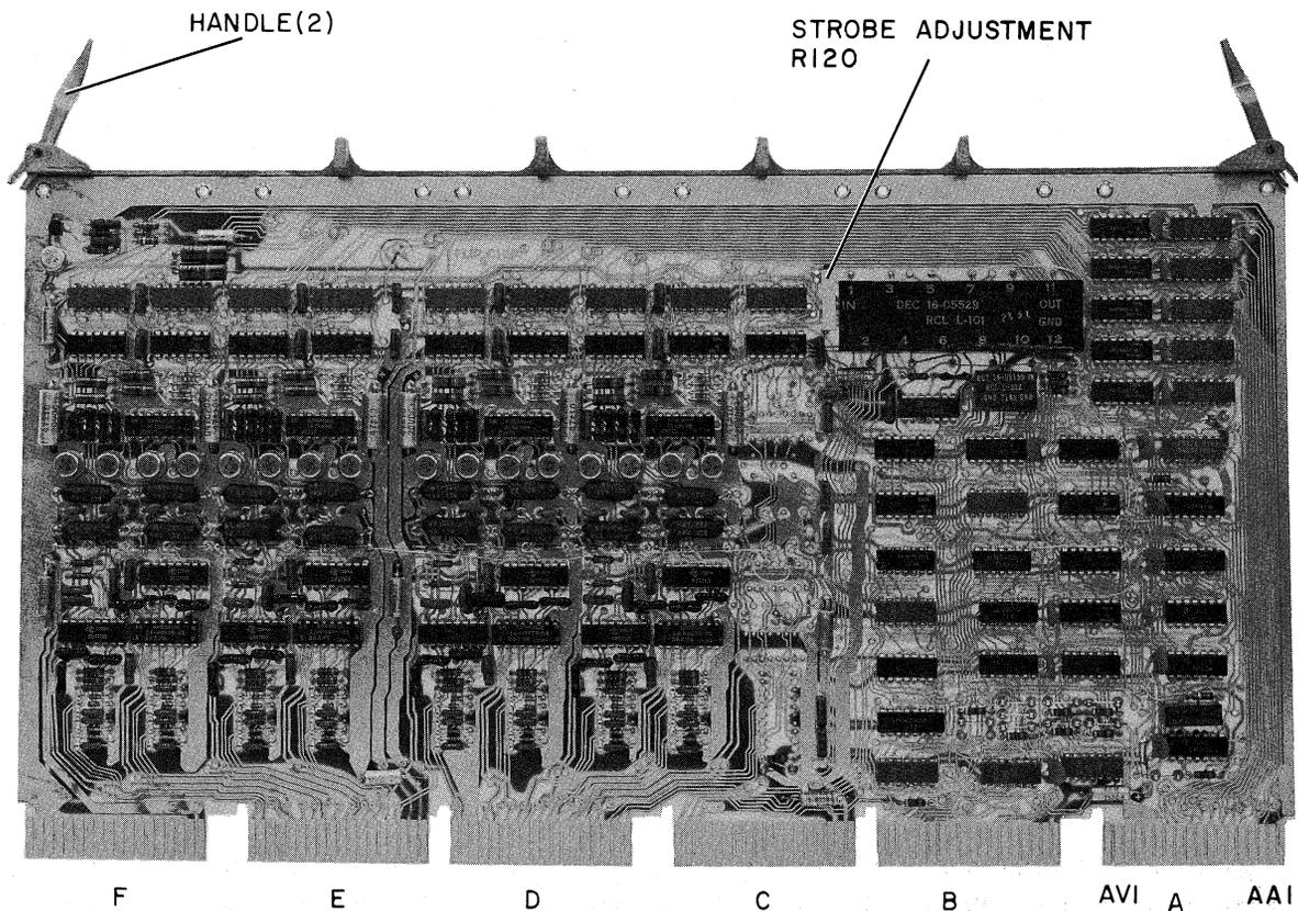
Figure 3-1 Component Side of Control Module G110
