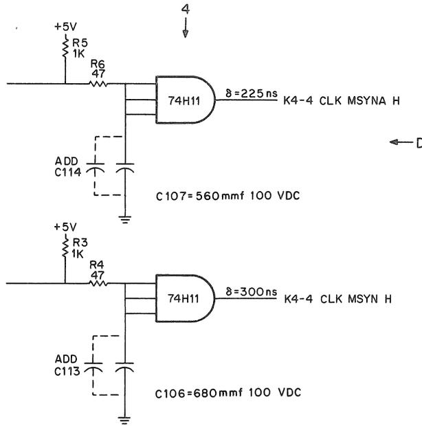
Figure 4-6 KD11-A Wiring Changes No. 6 and No. 7
