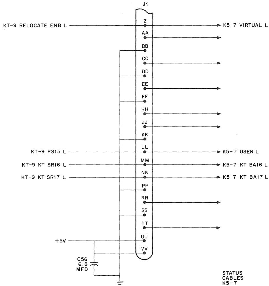
Figure 4-14 Console MM Enable Hooks In KD11-A
