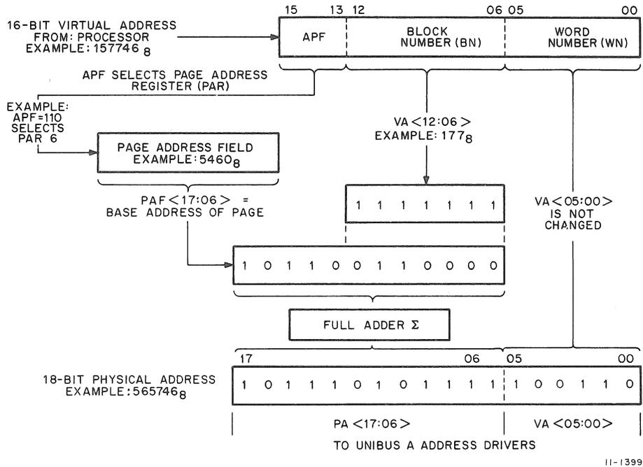
Figure 2-3 Construction of an 18-Bit Physical Address
