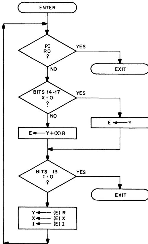
Figure 2-9 Effective Address Calculation
