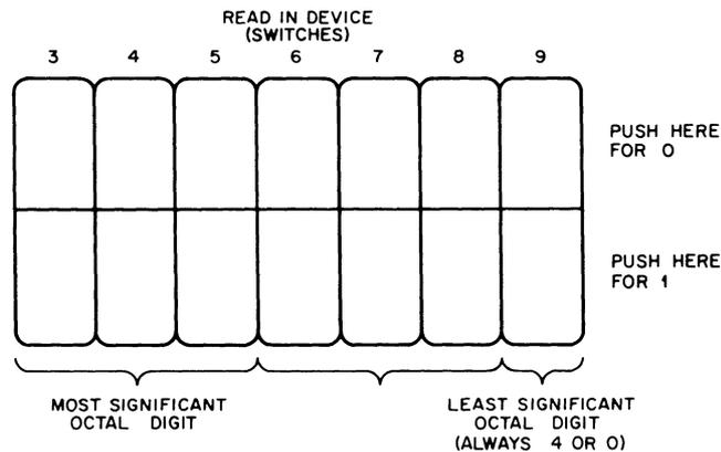
Figure 3-8 READIN DEVICE Switches
