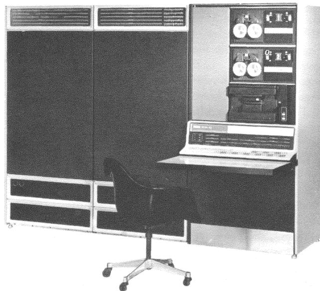
Figure 1-1 PDP-10 General Purpose Computer
