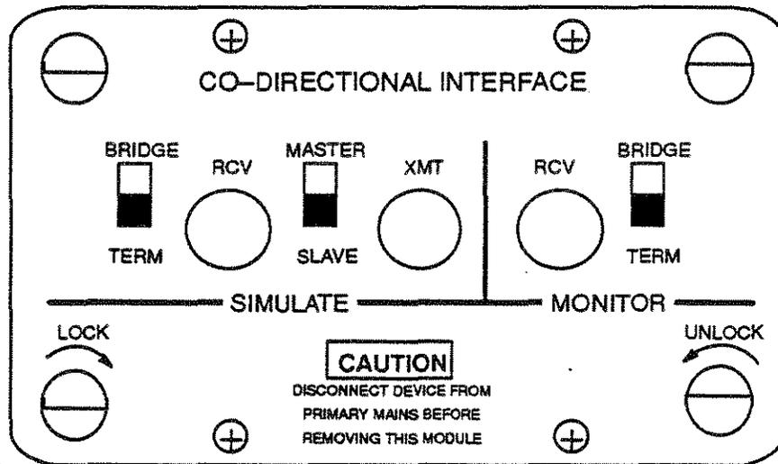
In simulate mode, the Co-Directional interface uses both the transmitter and receiver. In this mode, the Co-Directional interface module must be configured as a DTE. The Master/Slave switch selects the transmitter clock source used by the Co-Directional interface, as follows:
