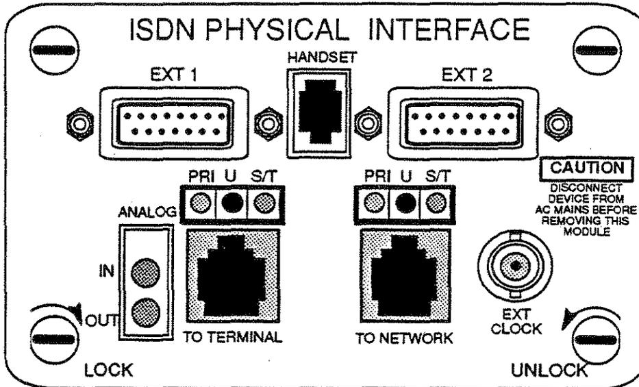
The EXT1 and EXT2 connectors are 15-pin, D-subminiature females, DA15S type. The figures below give the pinouts for these bi-directional connectors. All signals are standard RS422 voltage levels.
