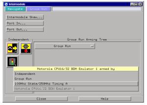
The emulation module is now set to stop the processor when the logic analyzer triggers.
