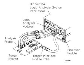
• Through an HP E2480A analysis probe, which provides a direct connection to the debug port pins.
