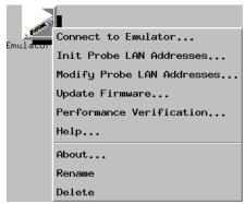
**3** Enter the emulation probe's LAN name or IP address and select the **Connect to Emulator** button.
