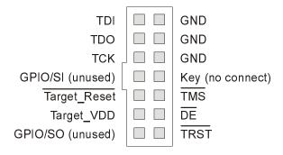
The connector on the target system should be placed as close as possible to the processor to ensure signal integrity.
