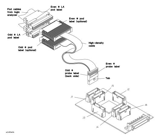
Connecting High-Density Cables to the Analysis Probe
