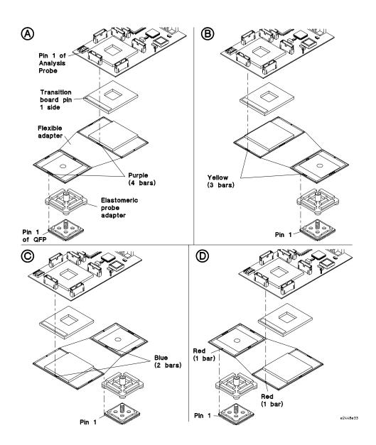
240-pin QFP Probe Adapter Rotation Diagram
