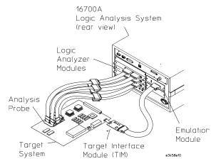
• Through an Agilent Technologies E2448A analysis probe, which provides a direct connection to the debug port pins.
