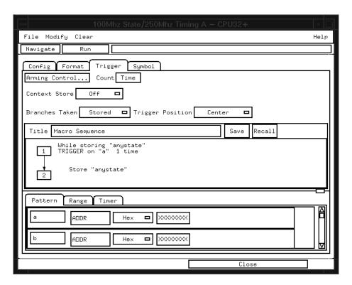
With the exception of Fastflush, all busses and signals defined in the Format menu are available for use in any single trigger term.
