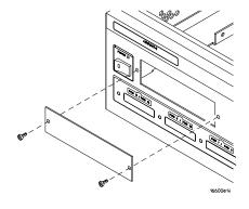
Chapter 6: Connecting and Configuring the Emulation Module **Installing the Emulation Module**
