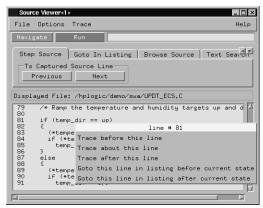
2 Select Trace→Enable - Break Emulator On Trigger.
