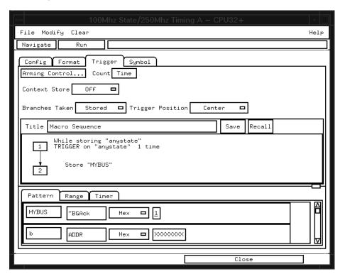
This allows other bus masters to gain control of the bus without having that activity captured by the logic analyzer.
