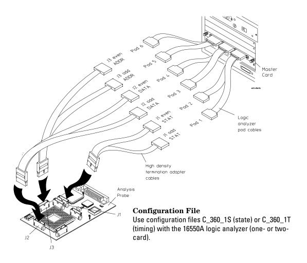
Expansion card connections for a two-card Agilent Technologies 16550A logic analyzer. Connection of J4, J5, and J6 is optional.
