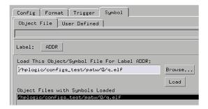
When you load object file symbols into a logic analyzer, a database of symbol/line number to address assignments is generated from the object file. The Symbol Selector dialog allows you to use a symbol in place of a hexadecimal value when defining trigger patterns, trigger ranges, and so on.
