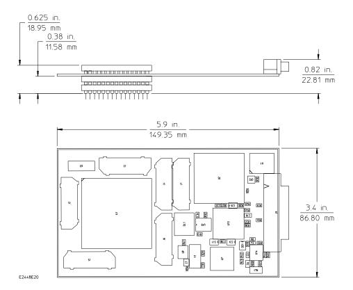
**Analysis Probe Circuit Board Dimension Diagram**
