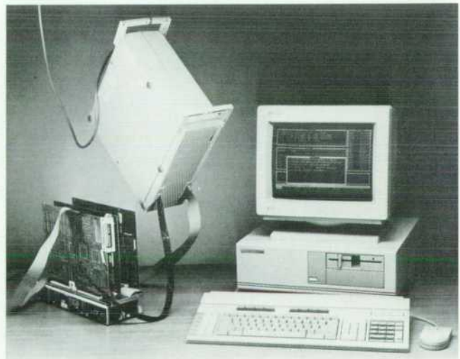
Fig. 5. Handles attach to the HP 64700 emulator chassis for standing or suspending the emulator close to the target system.
