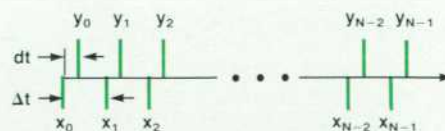
Fig. 1. Sampling of quadrature phase signals by waveform recorders. \epsilon = dt/\Delta t = 1/2 corresponds to the Redfield-Kunz case. dt = 100 ns corresponds to the HP Model 5180A.
