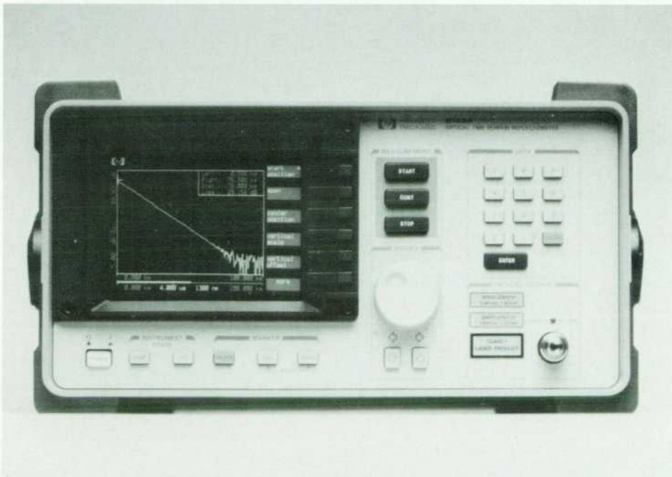
Fig. 1. The HP 8145A Optical Time-Domain Reflectometer makes one-port impulse response measurements of optical fibers and cables. It operates at 1300 nm, 1540 nm, or both, and has 0.01-dB power resolution, 1-m display resolution, and 200-km maximum range.
