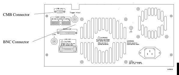
The location of the CMB and BNC connectors on the HP 64700 rear panel is shown in the following figure.
