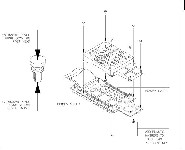
**2** Determine the placement of the emulation memory modules. Three types of modules may be installed: 256 Kbyte (HP 64171A/64172A), 1 Mbyte (HP 64171B/64172B), and 4 Mbyte (HP 64173A). Any of these types of modules may be installed in either memory slot on the probe (except 64748A which cannot accept HP 64173A).
