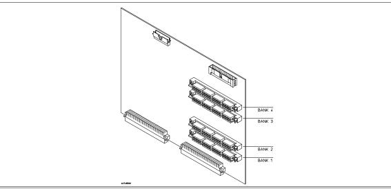
**2** To ensure correct installation of optional memory modules on the deep analyzer card, there is a cutout at one end of the memory modules so they can only be installed the correct way.
