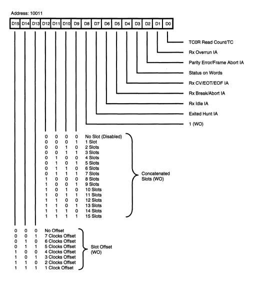
Figure 65c. Receive Interrupt Control Register (RICR)
