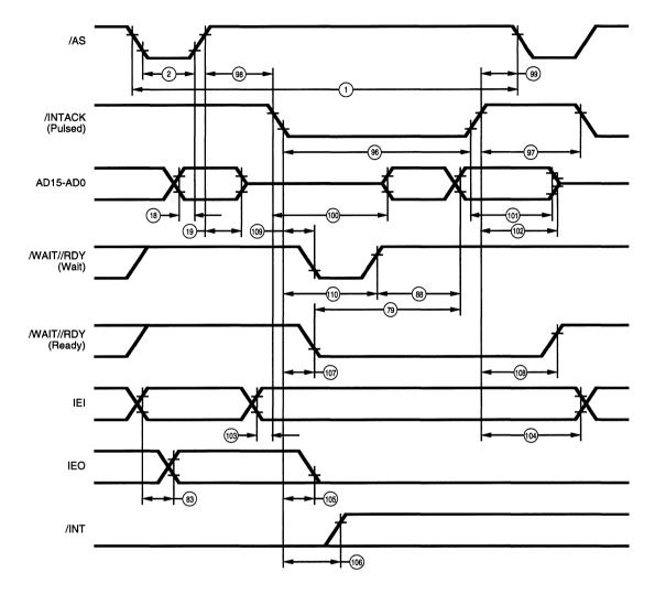
Figure 94. Multiplexed Pulsed Interrupt Acknowledge Cycle
