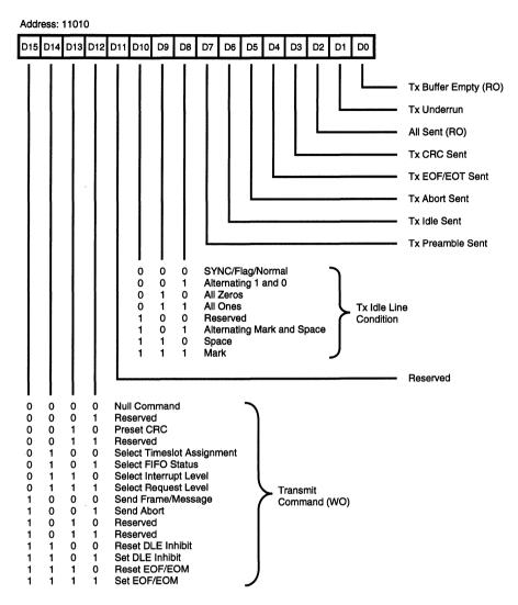
Figure 72. Transmit Command/Status Register (TCSR)
