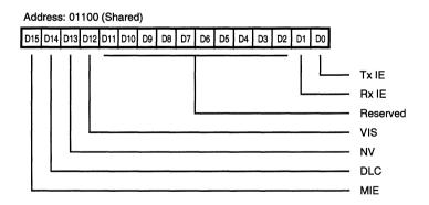
Figure 16. DMA Interrupt Control Register (DICR)
