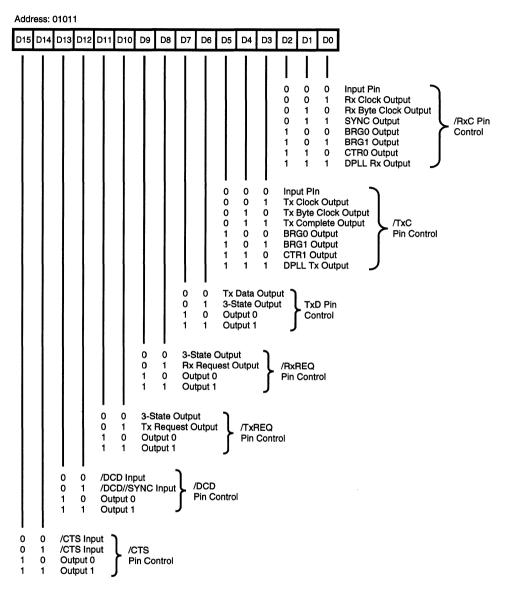
Figure 57. I/O Control Register (IOCR)
