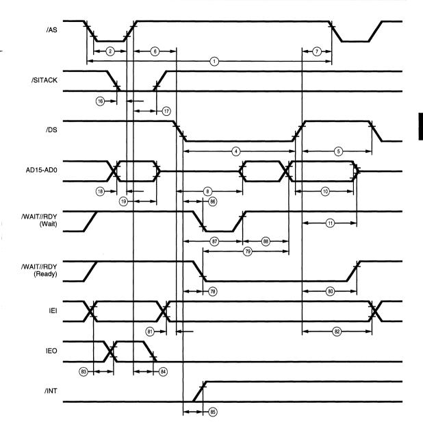
Figure 67. Multiplexed /DS Interrupt Acknowledged Cycle
