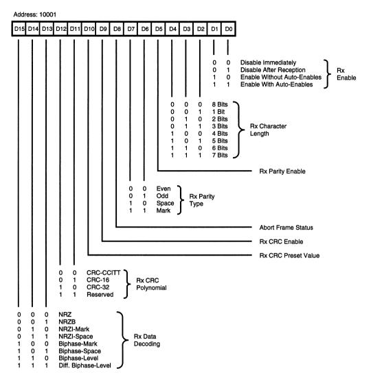
Figure 63. Receive Mode Register (RMR)
