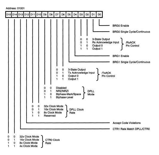
Figure 28. Hardware Configuration Register
