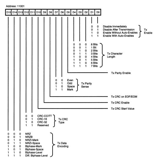
Figure 71. Transmit Mode Register (TMR)
