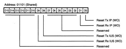
Figure 17. Clear DMA Interrupt Register (CDIR)
