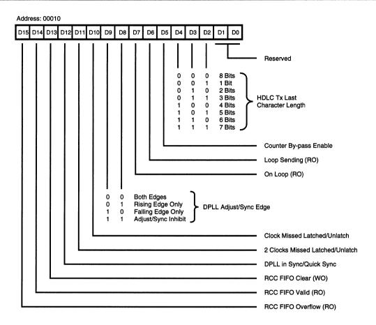
Figure 48. Channel Command/Status Register (CCSR)
