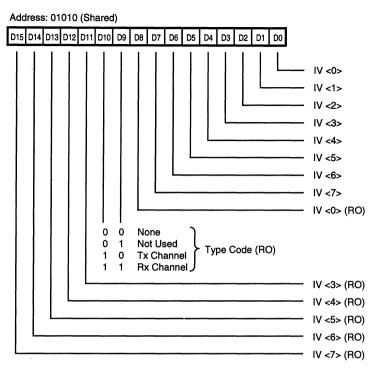
Figure 15. DMA Interrupt Vector Register (DIVR)
