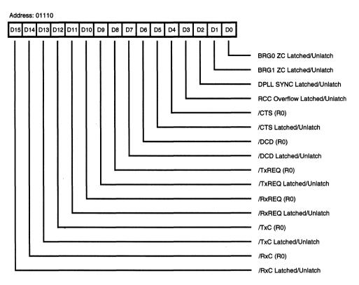
Figure 33. Miscellaneous Interrupt Status Register
