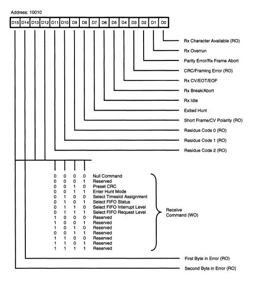
Figure 64. Receive Command Status Register (RCSR)
