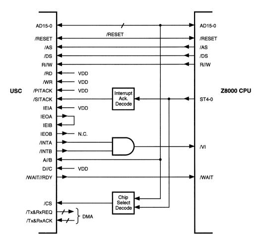
Figure 16. USC to Z8000 CPU Connection (Example)
