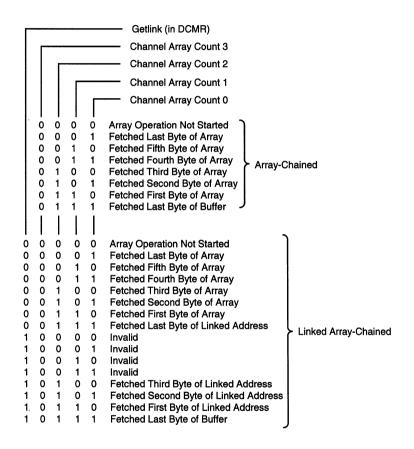
Figure 13b. Channel Array Count Bit Combinations
