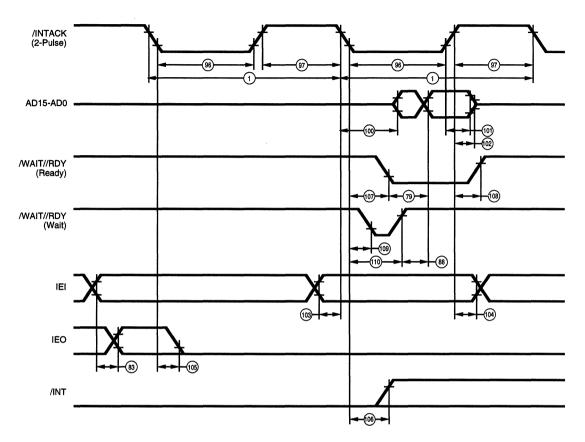
Figure 99. Non-Multiplexed Double-Pulse Intack Cycle
