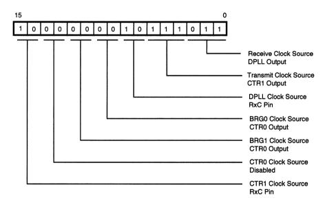
Figure 3. Clock Mode Control Register
