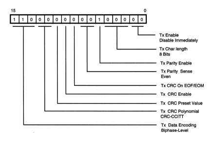
Figure 7. Transmit Mode Register
