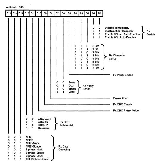
Figure 36. Receive Mode Register
