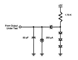
Figure 81. Standard Test Load
