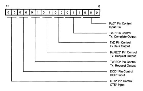
Figure 5. I/O Control Register
