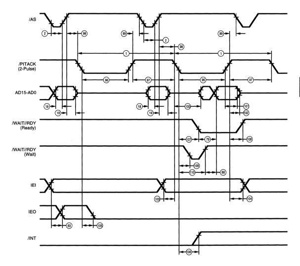
Figure 73. Multiplexed Double-Pulse Intack Cycle
