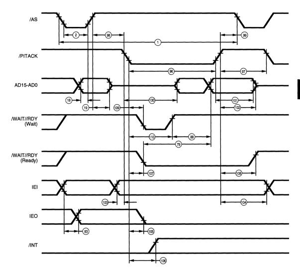
Figure 69. Multiplexed Pulsed Interrupt Acknowledge Cycle
