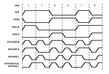
Figure 5. Data Encoding
