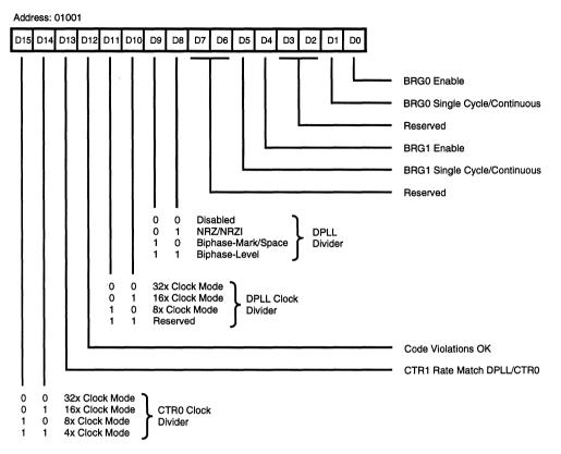
Figure 55. Hardware Configuration Register (HCR)
