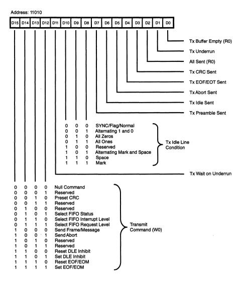
Figure 45. Transmit Command/Status Register
