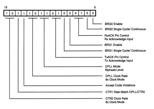
Figure 4. Hardware Configuration Register
