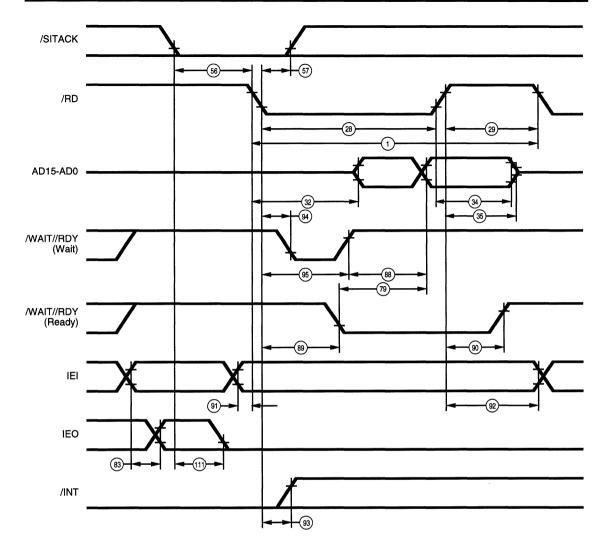
Figure 71. Non-Multiplexed /RD Interrupt Acknowledge Cycle
