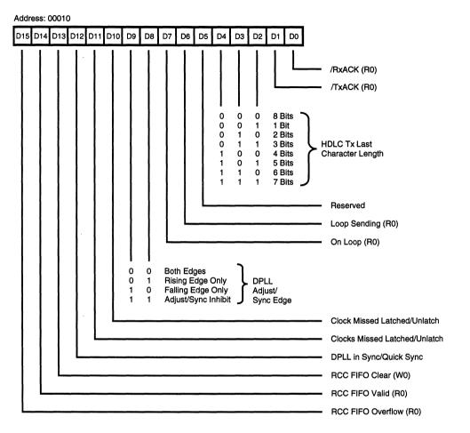
Figure 21. Channel Command/Status Register
