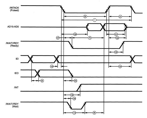
Figure 97. Non-Multiplexed Pulsed Interrupt Acknowledge Cycle
