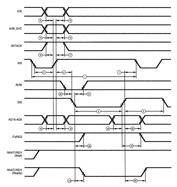
Figure 60. Multiplexed /DS Write Cycle
