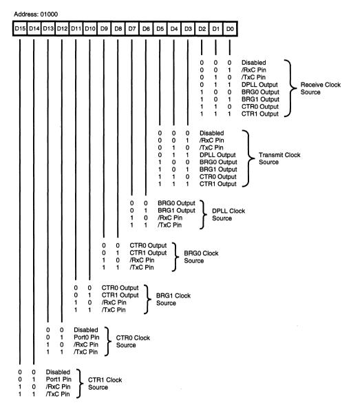
Figure 54. Clock Mode Control Register (CMCR)
