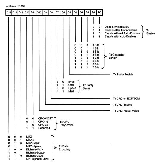
Figure 44. Transmit Mode Register
