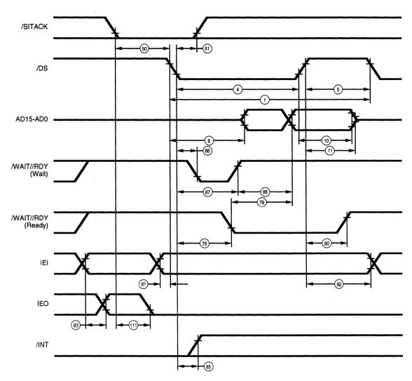
Figure 70. Non-Multiplexed /DS Interrupt Acknowledge Cycle
