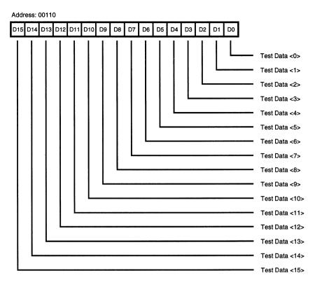
Figure 52. Test Mode Data Register (TMDR)
