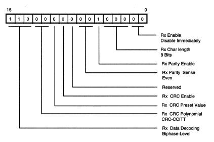
Figure 6. Receive Mode Register
