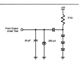
Figure 54. Standard Test Load
