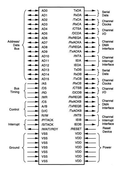
Figure 2. Pin Functions
