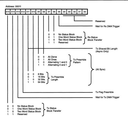
Figure 22. Channel Control Register
