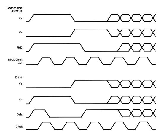
Figure 15. DPLL Idle Line Start-Up Requirements
