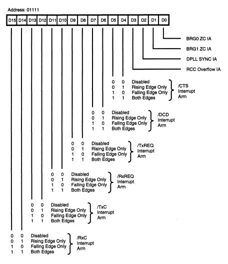
Figure 61. Status Interrupt Control Register (SICR)
