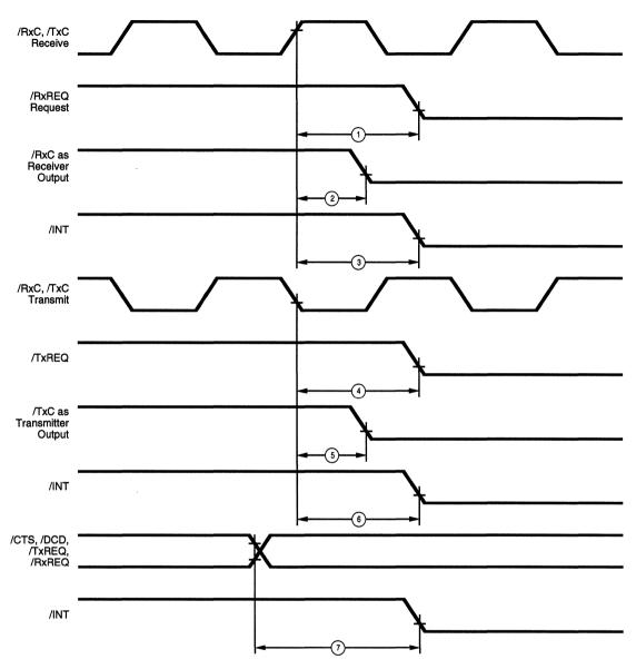
Figure 106. Z16C32 System Timing
