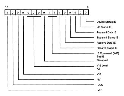
Figure 12. Interrupt Control Register
