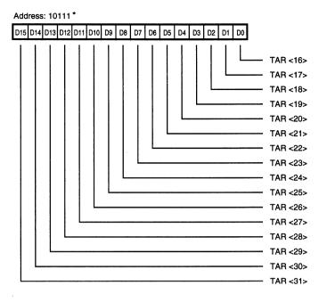
Figure 22. Tx/Rx Address Register (Upper) (TARU)/(RARU)
