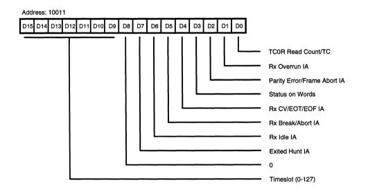
Figure 65b. Receive Interrupt Control Register (RICR)
