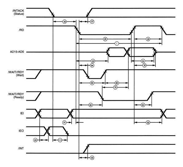
Figure 96. Non-Multiplexed /RD Pulsed Interrupt Acknowledge Cycle
