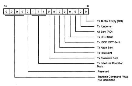
Figure 11. Transmit Command/Status Register
