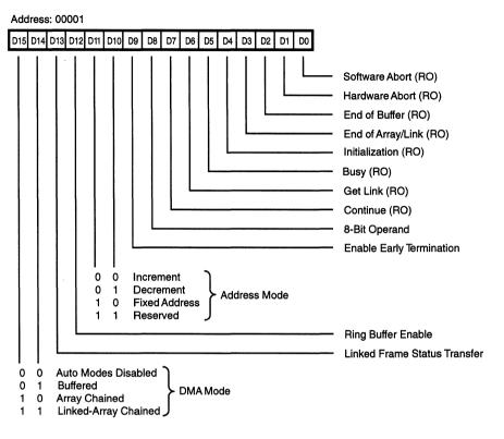
Figure 9. Tx/Rx DMA Mode Register (TDMR) (RDMR)
