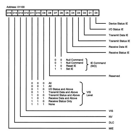
Figure 58. Interrupt Control Register (ICR)
