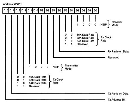
Figure 17. Channel Mode Register, NBIP Mode
