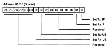
Figure 18. Set DMA Interrupt Register (SDIR)
