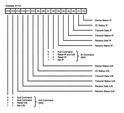
Figure 32. Daisy-Chain Control Register
