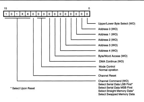
Figure 13. Channel Command/Address Register
