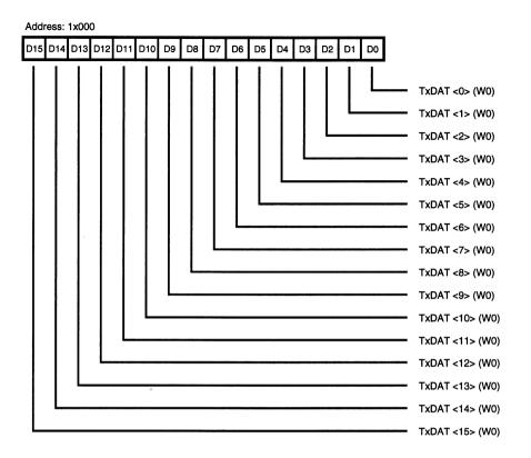
Figure 43. Transmit Data Register
