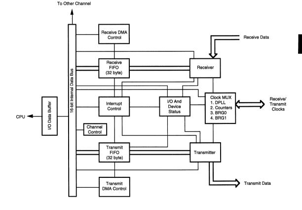
Figure 2. Z16C30 Universal Serial Controller
