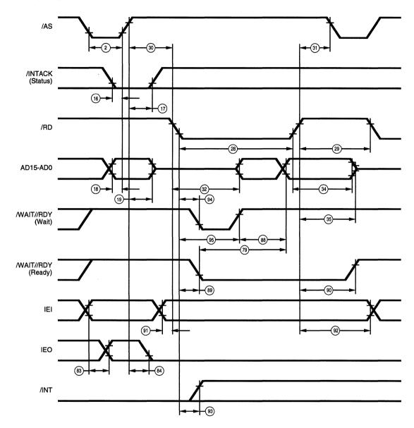
Figure 93. Multiplexed /RD Interrupt Acknowledge Cycle
