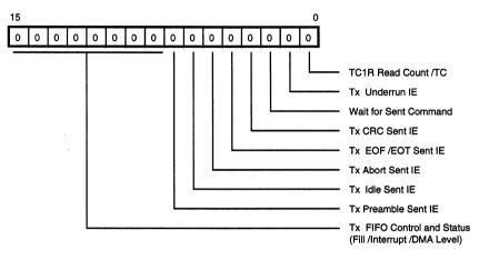
Figure 10. Transmit Interrupt Control Register
