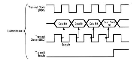
Note: /Transmit Clock Pin of USC is Programmed to be used as a Signal to Flag the End of Transmit.
