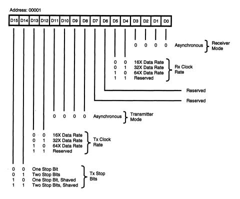
Figure 9. Channel Mode Register, Asynchronous Mode
