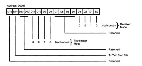
Figure 11. Channel Mode Register, Isochronous Mode
