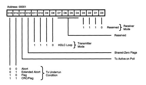
Figure 20. Channel Mode Register, HDLC Loop Mode
