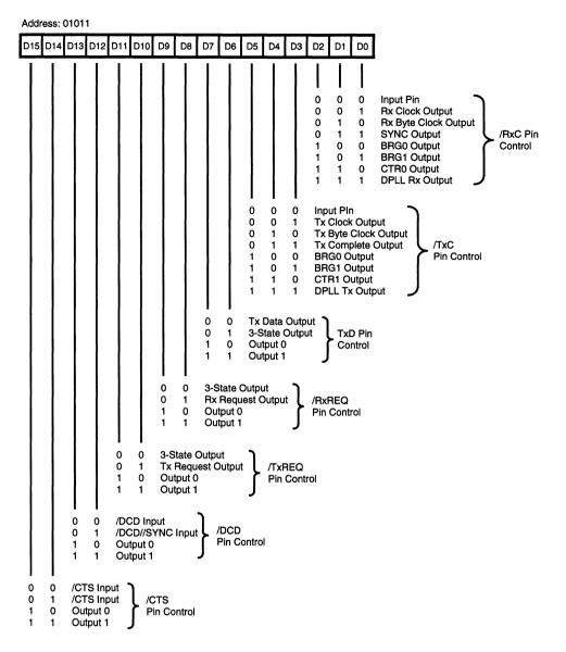
Figure 30. I/O Control Register
