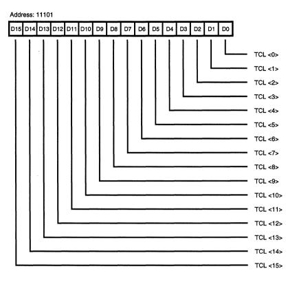
Figure 75. Transmit Count Limit Register (TCLR)
