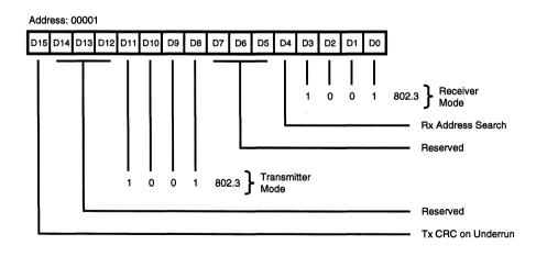
Figure 18. Channel Mode Register, 802.3 Mode
