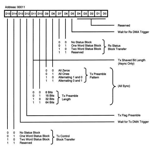
Figure 49. Channel Control Register (CCR)
