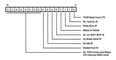
Figure 9. Receive Interrupt Control Register
