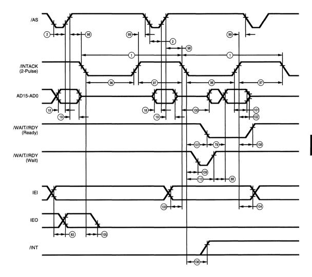
Figure 98. Multiplexed Double-Pulse Intack Cycle
