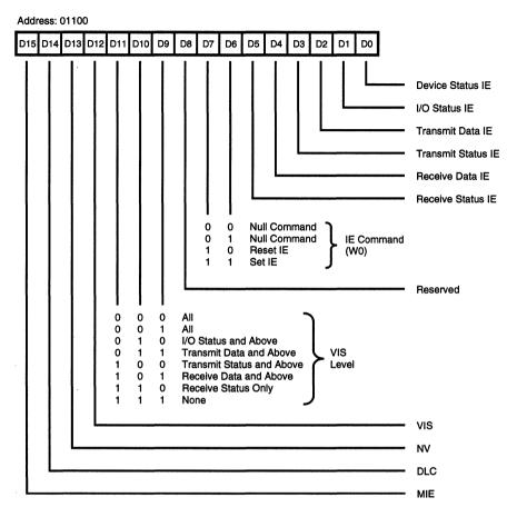
Figure 31. Interrupt Control Register
