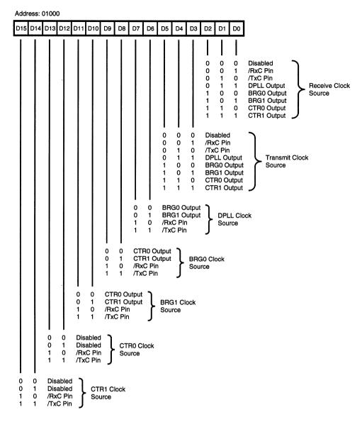
Figure 27. Clock Mode Control Register
