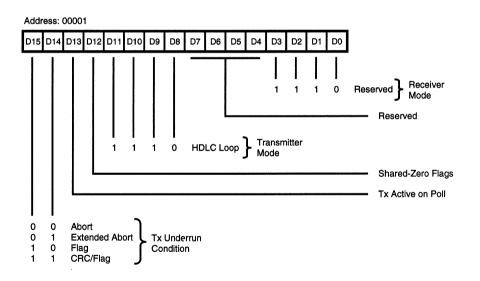
Figure 47. Channel Mode Register, HDLC Loop Mode
