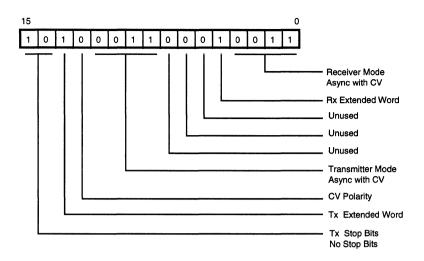
Figure 8. Channel Mode Register
