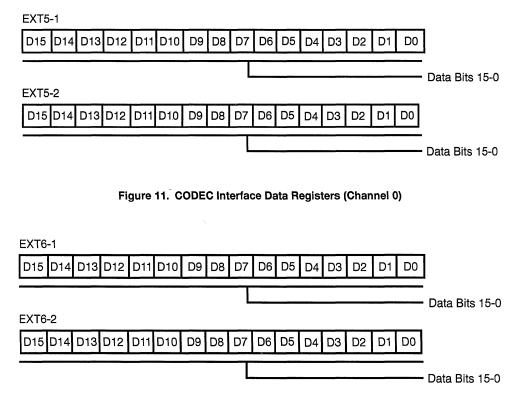
Figure 12. CODEC Interface Data Registers (Channel 1)
