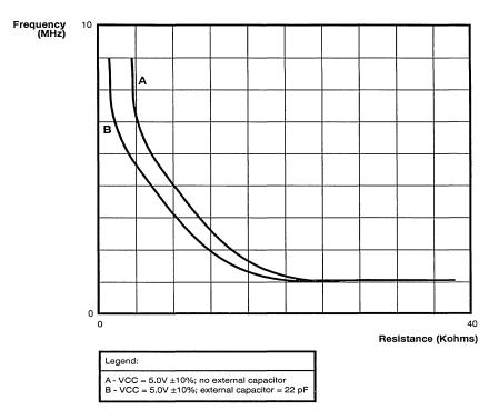
Figure 62. Typical Frequency vs RC Resistance
