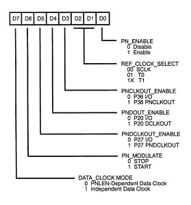
Figure 18. PN Modulator Control Register (PNCON)
