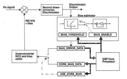
Figure 5. AFC Loop and Processor Control
