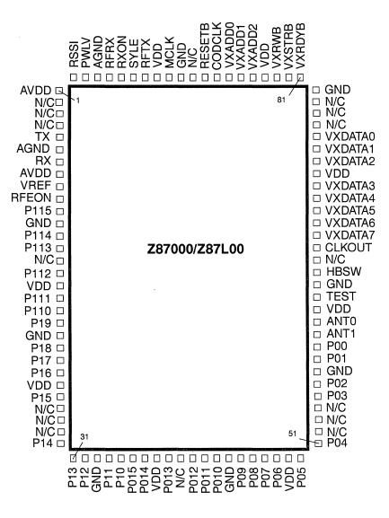
Figure 4. 100-Pin QFP Pin Configuration
