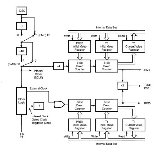
Figure 14. Counter/Timer Block Diagram
