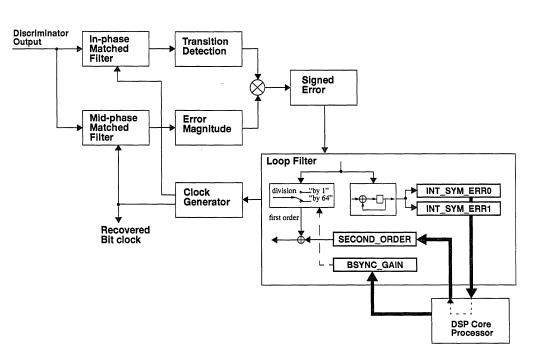
Figure 6. Bit Synchronizer Loop and Processor Control
