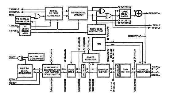
Figure 10. Transmitter and Receiver Test Points
