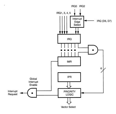
Figure 15. Interrupt Block Diagram
