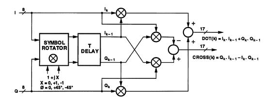
Figure 8. DPSK Demodulator I and Q Channel Processing
