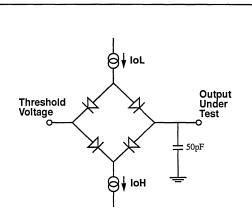
Figure 4. Test Load Diagram
