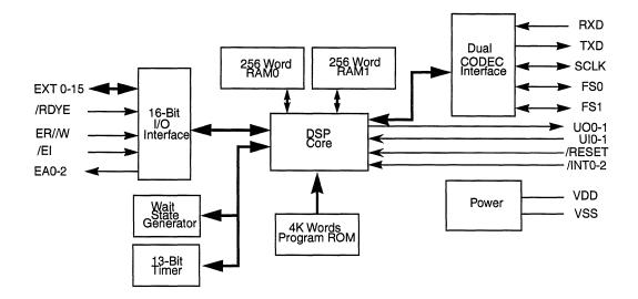
Figure 1. Z87010 Functional Block Diagram
