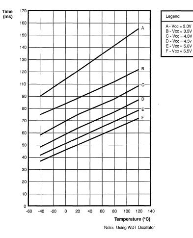
Figure 60. Typical 25 ms WDT Setting vs Temperature
