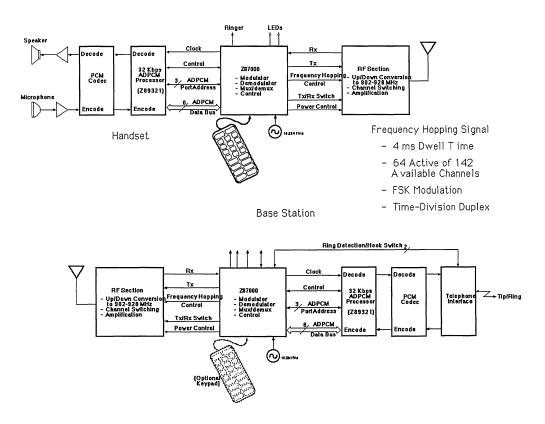
Figure 4. Z87000 Cordless Phone Transceiver/Controller
