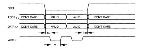
Figure 3. Microprocessor Interface Timing
