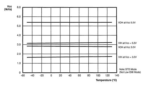
Figure 54. Typical  $V_{\text{OH}}, V_{\text{IH}}$  vs Temperature
