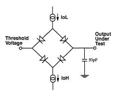
Figure 5. Test Load Diagram
