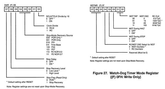
Figure 26. Stop-Mode Recovery Register ((F) 0BH: Write Only) 3
