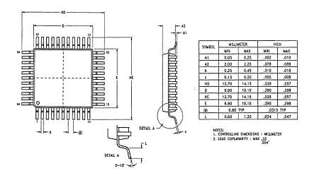
Figure 4. 44-Pin QFP Package Diagram
