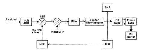
Figure 2. Demodulator Block Diagram
