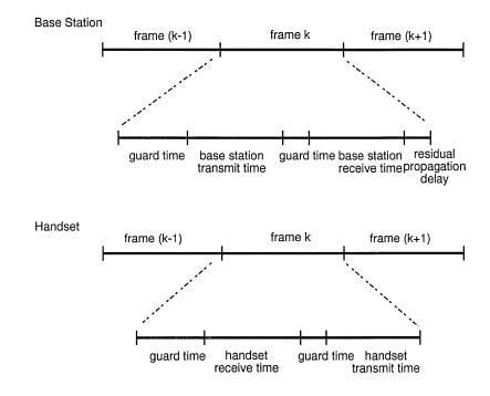
Figure 1. TDD Frame Structure
