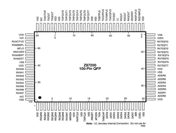
Figure 2. Z87200 100-Pin PQFP Pin Description
