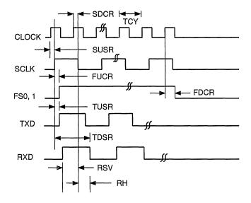
Figure 8. CODEC Interface Timing
