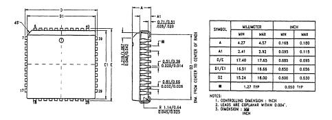
Figure 3. 44-Pin Lead PLCC Package Diagram
