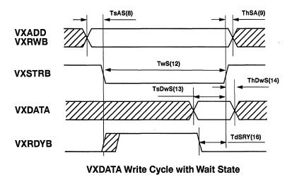
Figure 9. Read/Write Cycle Timing with Wait State
