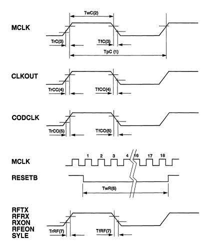
Figure 7. Transceiver Output Signal
