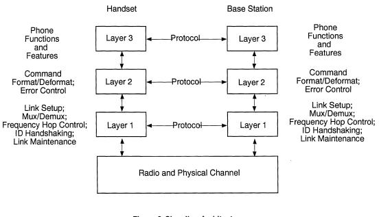
Figure 6. Signaling Architecture
