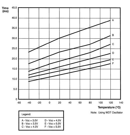
Figure 58. Typical 5 ms WDT Setting vs Temperature
