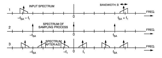
Figure 12. Direct I.F. Sampling Mode with I.F. Frequency (f<sub>SA</sub>+f<sub>1</sub>) > Sampling Frequency f<sub>SA</sub>
