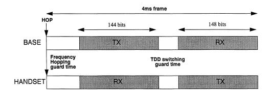
Figure 1. Basic Time Duplex Timing
