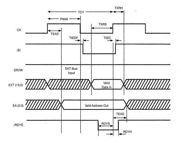
Figure 6. Read From External Device Timing
