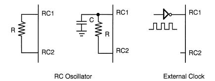
Figure 16. RC Oscillator Configuration
