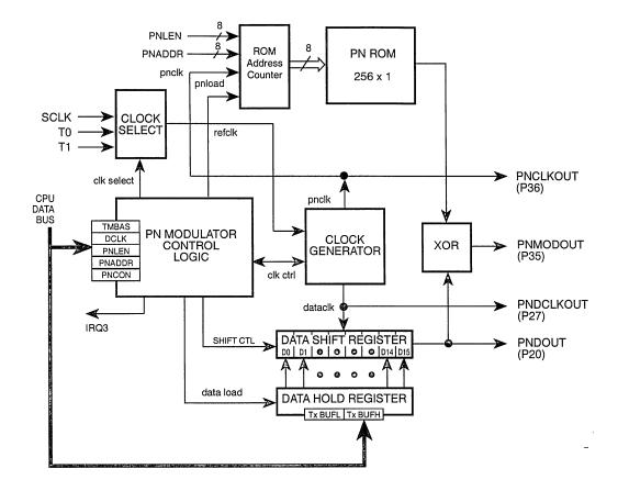
Figure 17. Z87100 PN Modulator Conceptual Block Diagram
