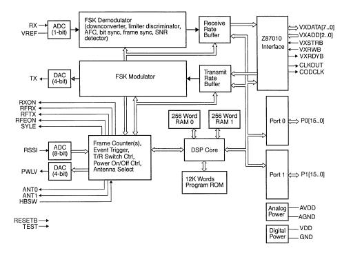
Figure 2. Z87000 Functional Block Diagram
