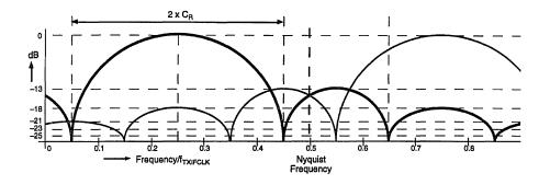
Figure 19. Spectrum of DDS Modulated at 0.4 x f<sub>RXIFCLK</sub> When Carrier Frequency is set to 0.25 x f<sub>RXIFCLK</sub>
