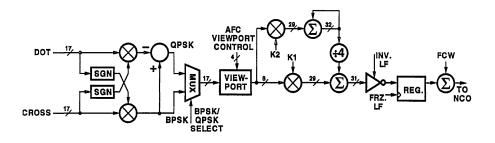
Figure 9. Frequency Discriminator and Loop Filter Detail
