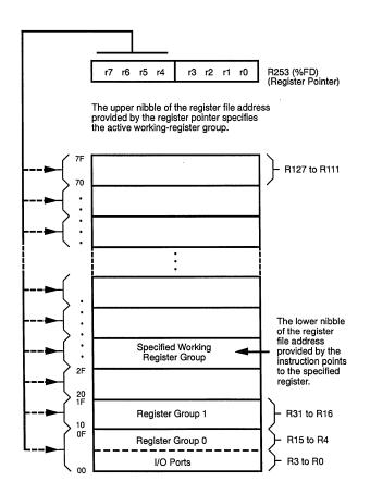
Figure 13. Register Pointer
