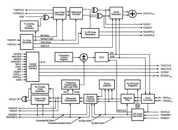
Figure 1. Z87200 Block Diagram
