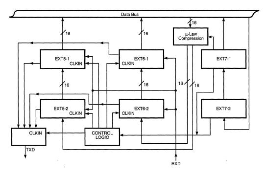
Figure 9. CODEC Interface Block Diagram
