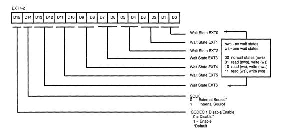
Figure 14. Wait/State/CODEC Interface Control Register
