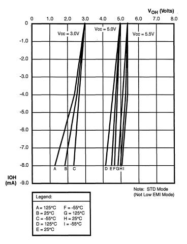
Figure 55. Typical  $V_{OH}$  vs  $I_{OH}$  Over Temperature
