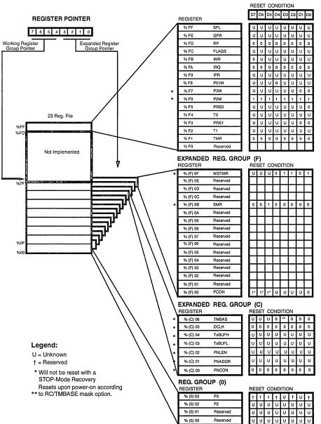
Figure 11. Expanded Register File Architecture
