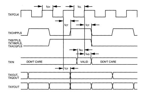
Figure 4. Transmitter Input/Output Timing
