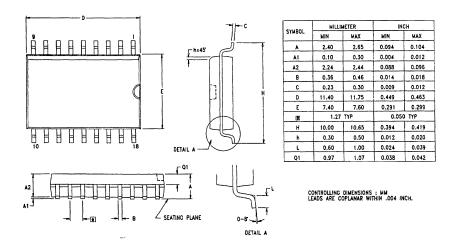
Figure 2. 18-Pin SOIC Package Diagram
