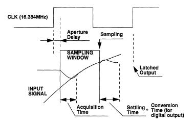
Figure 6. 1-Bit ADC Definition of Terms
