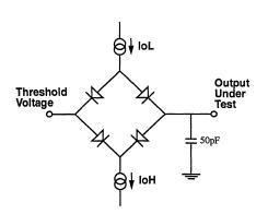
Figure 3. Test Load Configuration
