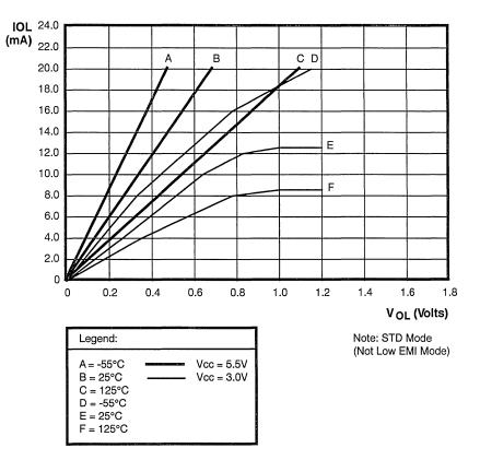
Figure 56. Typical  $I_{\text{OL}}$  vs  $V_{\text{OL}}$  Over Temperature
