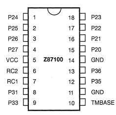
Figure 2. 18-Pin DIP/SOIC Pin Configuration
