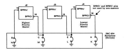
Figure 8–12. Serial DMA Priority
