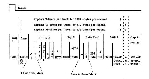
Figure 6-2. 431 Soft-sectored Winchester Disk Format
