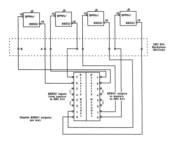
Figure 8-13. Parallel DMA Priority
