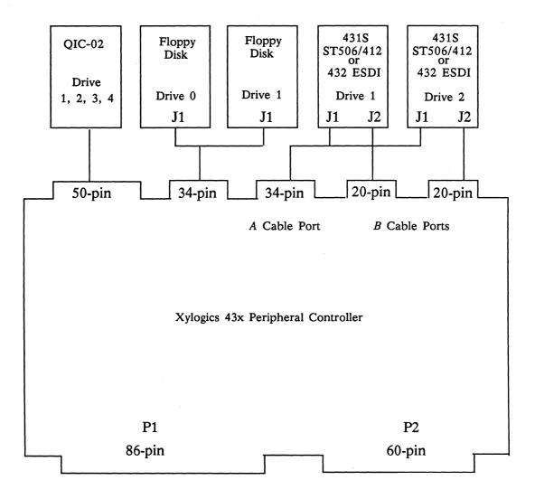
Figure 8-14. Multiple Drive Connection Diagram
