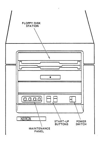
Figure 2. The Front of the Server Processor
