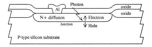
Figure 3. An NMOS Photo-Diode.
