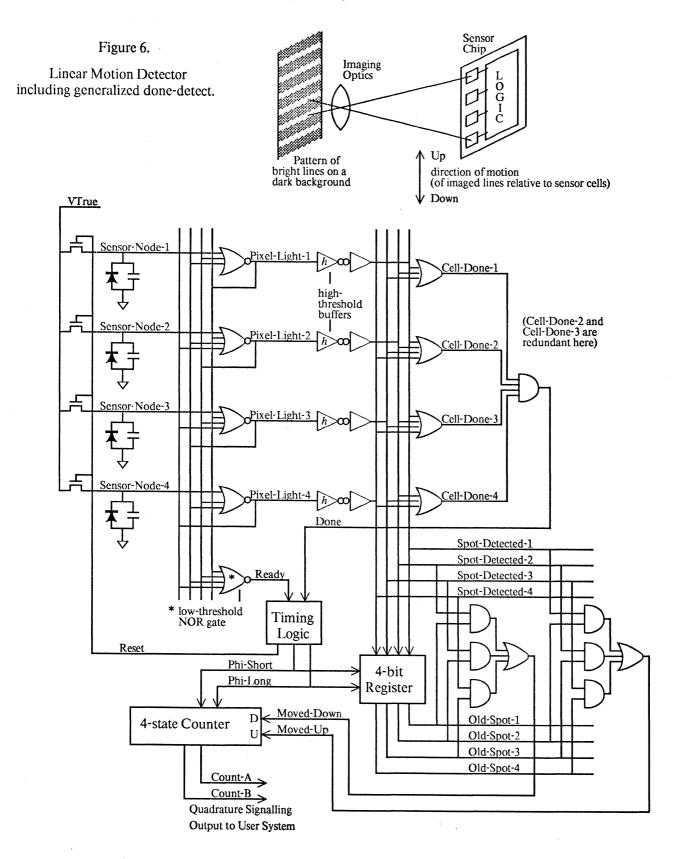
Note that we do not use the inhibition NOR gate output itself for done-detection, but a buffered version of it after a high threshold buffer (inverter pair); this is the easiest way to prevent false done-detection during a metastable condition [Seitz 1980]. The buffered signal is not used for inhibition, since that would make it participate in the metastable condition, and because the extra delay would cause oscillatory metastable states.
