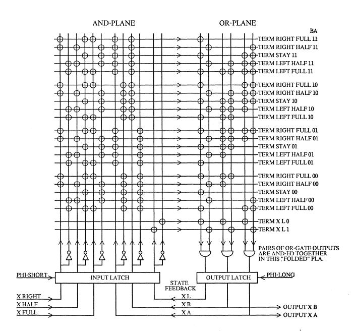
CIRCLES INDICATE GATE INPUTS TO AND-GATES (TERMS) AND OR-GATES (OUTPUTS). LOGIC EQUATIONS CAN BE READ OFF BY INSPECTION.
