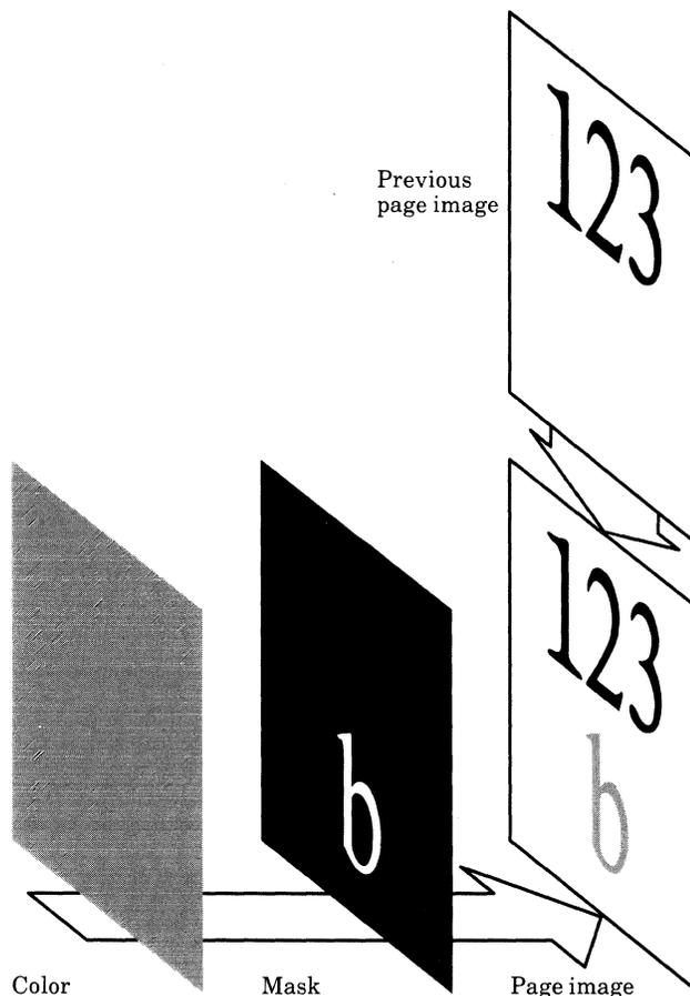
Figure 4.1 The imaging model; application of a mask operator
