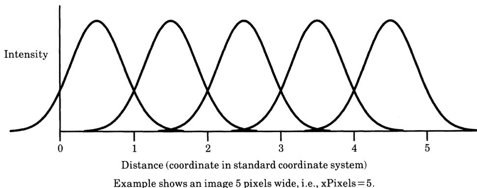
Figure 4.3 Pixel intensity profiles
