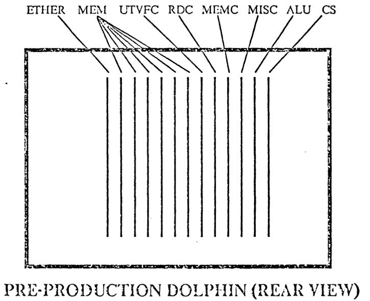
Figure 2-1: Backplane configuration for pre-production and production Dolphins
