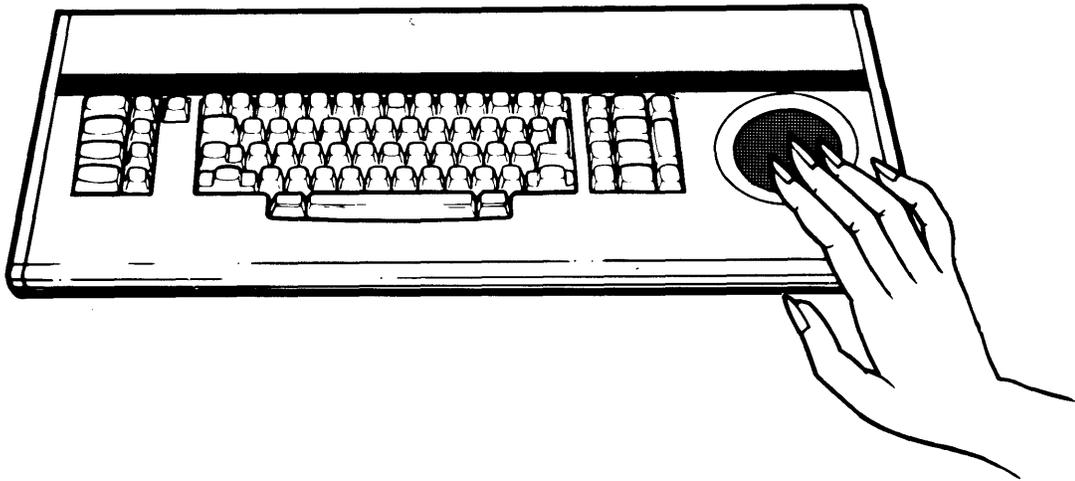
The **CAT** is the circular pad located to the right of the keyboard. It's activated by the touch of your fingers and is used to move the cursor around on the screen. The cursor moves in the same direction that your fingers do on the pad. In other words, if you put your fingers at the bottom of the pad, the cursor will move to the bottom of the screen.
