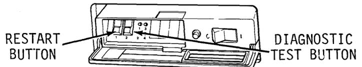
During the test, you will see a variety of test patterns on the screen and different numbers in the display on the diagnostic panel. At the end of the test --
