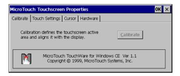
The **Calibrate** properties sheet has one command button. Click on the **Calibrate** command button to begin the calibration process. A white screen with a single crosshair in the upper left hand corner displays:
