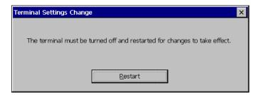
This dialog box contains the **Restart** command button. The terminal must be restarted in order for your new settings to take effect. Click on **Restart** to restart the terminal. The **Winterm Connection Manager** displays. See "Connections Management" for detailed information about configuring and making terminal connections.
