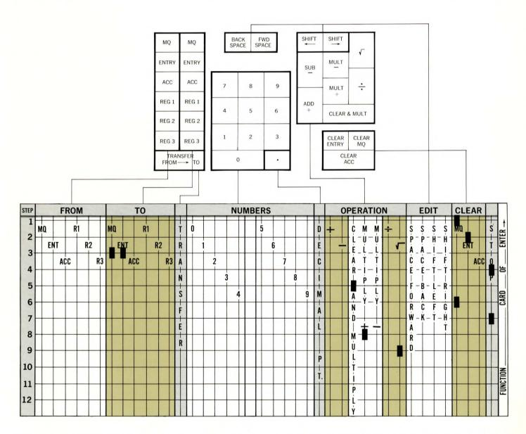
To program problems requiring more steps than are provided for on each card, you continue programming on additional cards. When you feed the prepared cards into PAC, the *Scientific* operates automatically until a "Stop" is reached. You then insert the variable through the keyboard, and automatic operation is resumed until another variable is required or the problem is completed.
