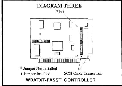
Most SCSI devices used by the FASST controller have keyed connectors and the cable can only be plugged in one way. If, however, the SCSI device
