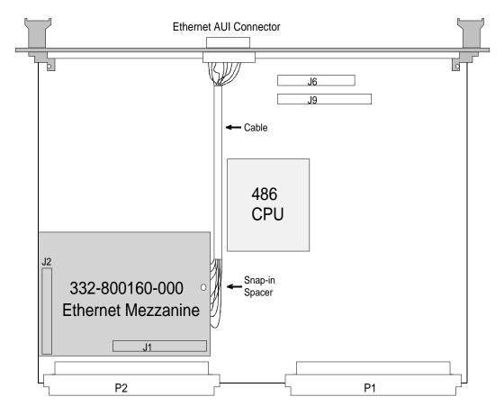
Figure A-1 Location of the Ethernet Mezzanine
