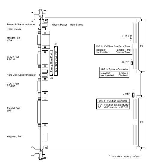
Figure 2-1 I/O Port and Jumper Locations
