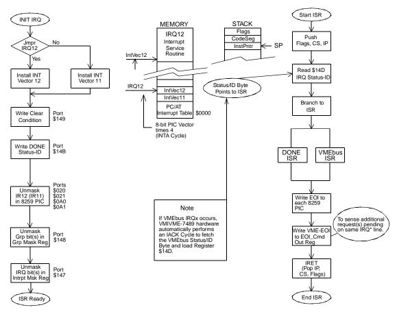
Figure 4-5 Interrupt Response Flow Chart
