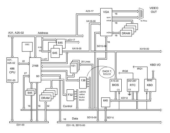
Figure 1-2 VMIVME-7486 Partial Block Diagram
