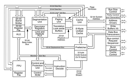
Figure 3-1 80486 CPU Block Diagram
