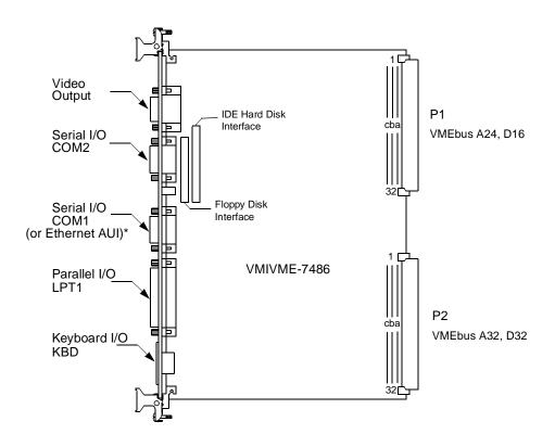
\* Serial port COM1 is unavailable if the Ethernet Mezzanine option is ordered, since the Ethernet AUI connector replaces the COM1 connector. See Appendix A, *Ethernet Option* on page 99 for Ethernet Mezzanine option details.
