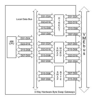
Figure 4-4 80486-to-VMEbus Data Byte Lanes
