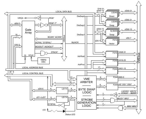
Figure 4-1 VMIVME-7486 VMEbus Interface Block Diagram
