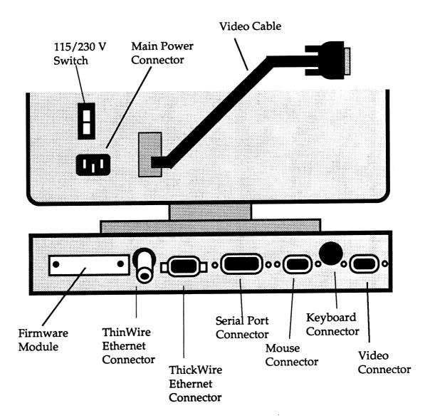
Figure 2: Rear View of the X-19
