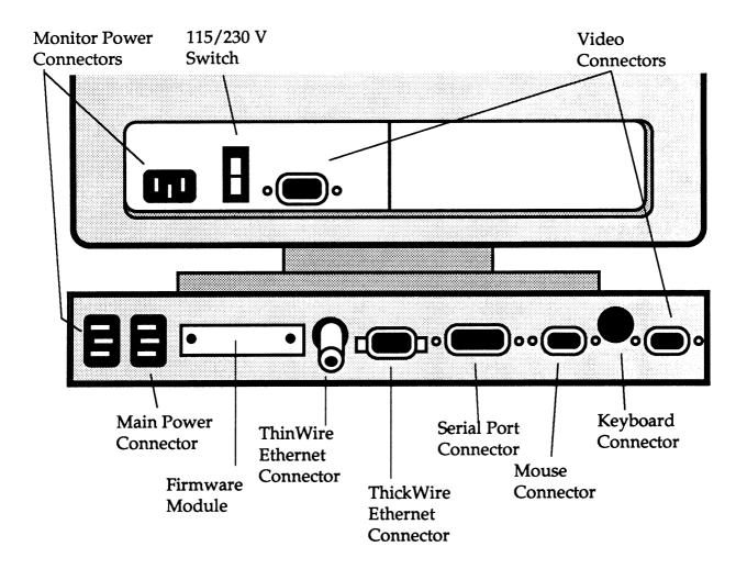
Figure 3: Rear View of the X-19 Turbo
