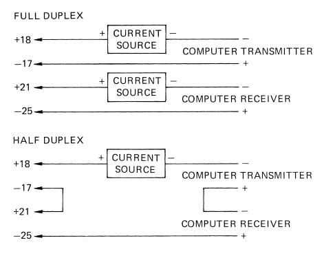
Figure 5-2 Current Loop Connections
