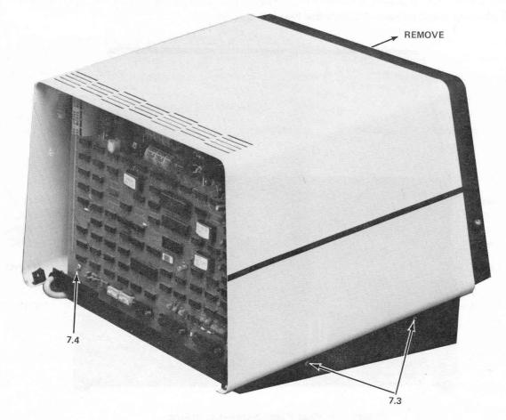
Figure 7-2 Top Cover Removal
