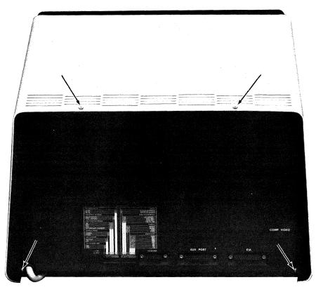
Figure 7-1 Rear Panel Screw Locations
