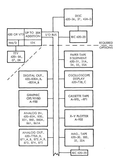
EXTENDED BASIC expands on the BASIC language with special commands to control an external data acquisition and process control system, as shown in the diagram. In addition, directives have been included to allow the creation and control of files stored on a rotating memory device, and to facilitate chaining of program overlay segments.
