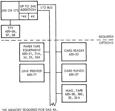
AK MEMORY REQUIRED FOR DAS 8A, DASMR WILL RUN IN 8K MEMORY WITH LIMITED CAPABILITIES. 12K IS RECOM-MENDED FOR MOST APPLICATIONS.
