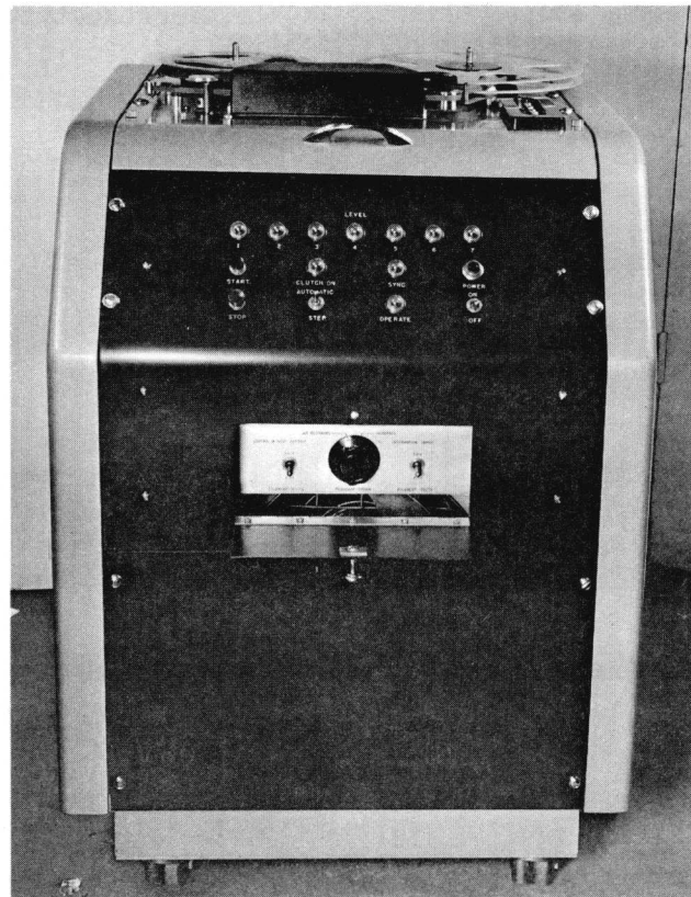
Magnetic Tape Input Reader
