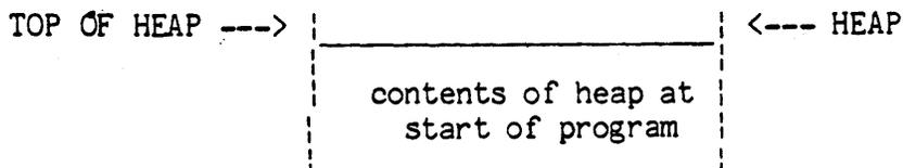
Once the program no longer needs the variable P^ and wishes to "release" this memory space to the system for other uses, it calls RELEASE which resets the top of heap to the address contained in the variable HEAP.
