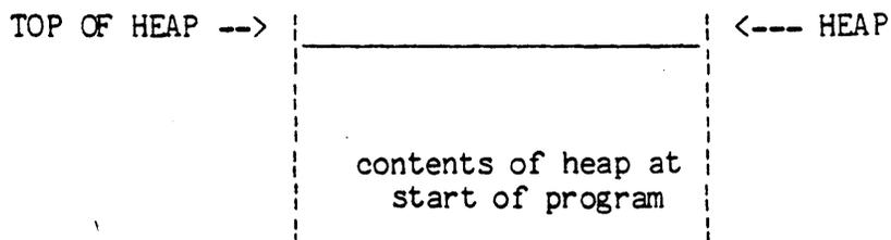
Next the program calls the standard procedure NEW and this results in a new variable P^ which is located in the heap as shown in the diagram below:
