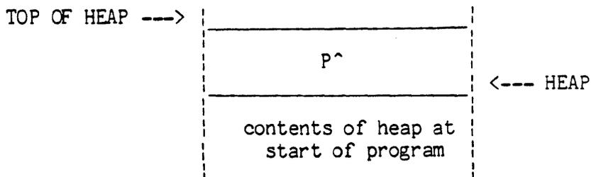
After the RELEASE the heap is as follows:
