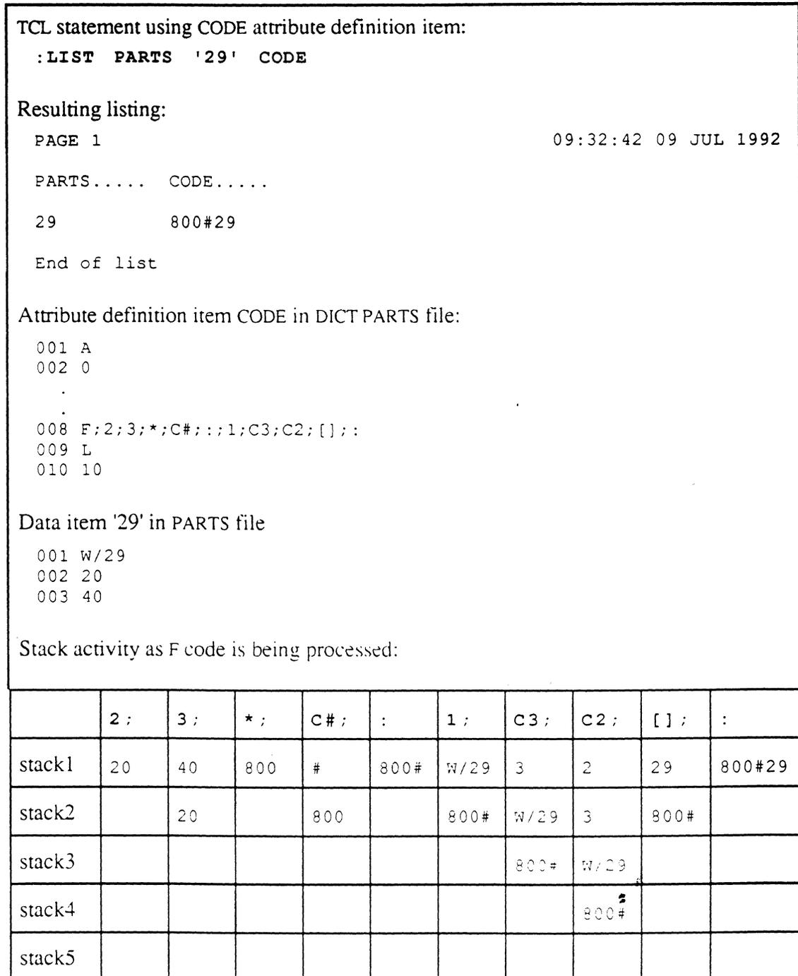
Figure 5-2. F-Code Stack Activity to Resolve F;2;3;\*;C#;;;1;C3;C2;[];;
