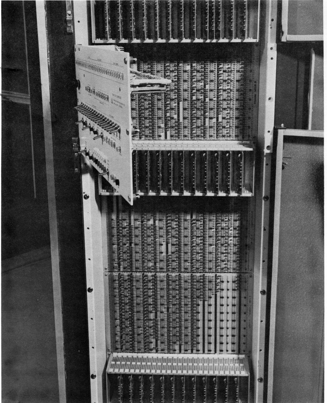
FIGURE A-1. FRONT VIEW - TRW-340 ARITHMETIC AND CONTROL UNIT
