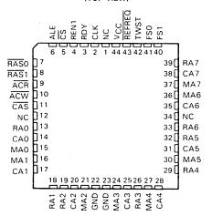
The controller contains a 16-bit multiplexer that generates the address lines for the memory device from the 16 system address bits and provides the strobe signals required by memory to decode the address. An 8-bit refresh counter generates the 256-row addresses required for refresh.
