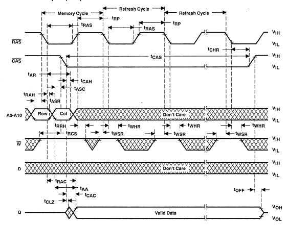
hidden refresh cycle (write) Refresh Cycle **Memory Cycle** Refresh Cycle t<sub>RP</sub> tRP -tRAS → tRAS → ۷ін RAS ٧ıL tCHR -- tCAS  $V_{1H}$ CAS  $v_{IL}$ tCAH **t**ASC <sup>t</sup>RAH tAR Don't Care Col A0-A10 <sup>t</sup>RRH - twhr twcs twsR **tWCR** tDHR tDS  $v_{\text{IH}}$  $V_{IL}$ νон HI-Z Q VOL
