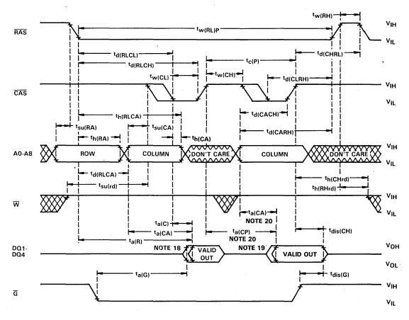
NOTES: 18. Output may go from high impedance to an invalid data state prior to the specified access time.
