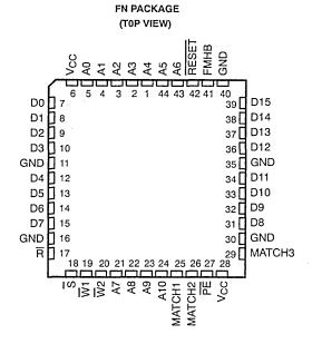
When  $\overline{S}$  is low and  $\overline{W}1$ ,  $\overline{W}2$ , and  $\overline{R}$  are high, the cache address comparator compares the contents of the memory location addressed by A0-A10 with the applied D0-D15 plus generated byte parity. An equality is indicated by a high level on the MATCH1, MATCH2, and MATCH3 outputs.
