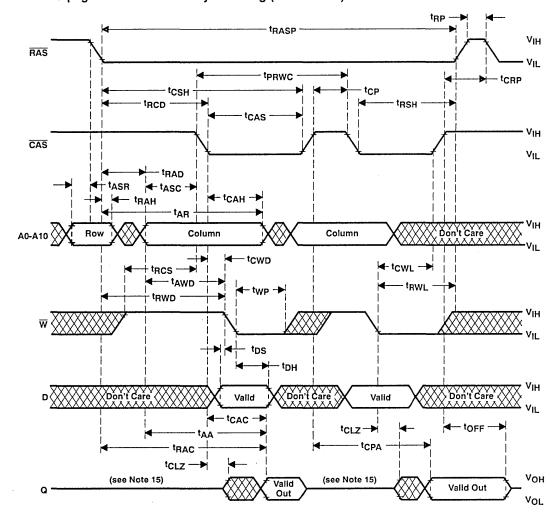
NOTES: 15. Valid data is presented at the output after all access times are satisfied. The output may go from three-state to an invalid data state prior to the specified access times as the output is driven when CAS goes low.
