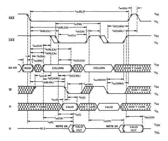
NOTES: 23. A read or a write cycle can be intermixed with read-modify-write cycles as long as the read and write timing specifications are not violated.
