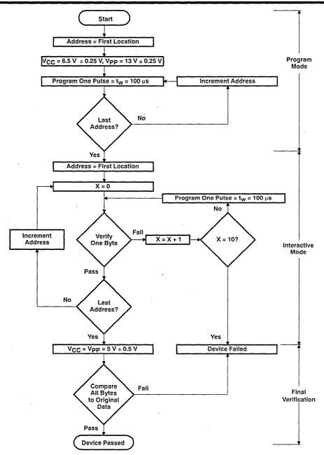
Figure 1. SNAP! Pulse Programming Flow Chart
