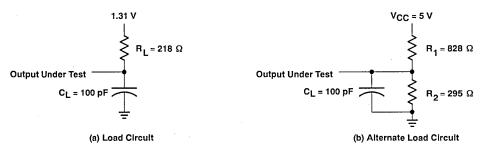
Figure 1. Load Circuits for Timing Parameters
