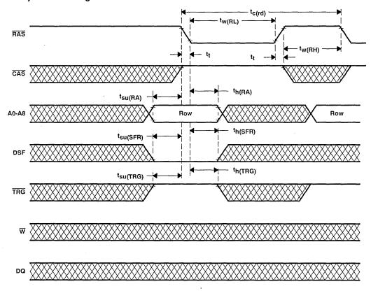
NOTE 29: In persistent write-per-bit function,  $\overline{W}$  must be high during the refresh cycles.
