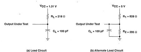
Figure 1. Load Circuits for Timing Parameters
