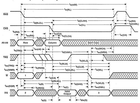
NOTE 24: See "Write Cycle State Table" for the logic state of "1", "2", and "3". Same logic as delayed write cycle.
