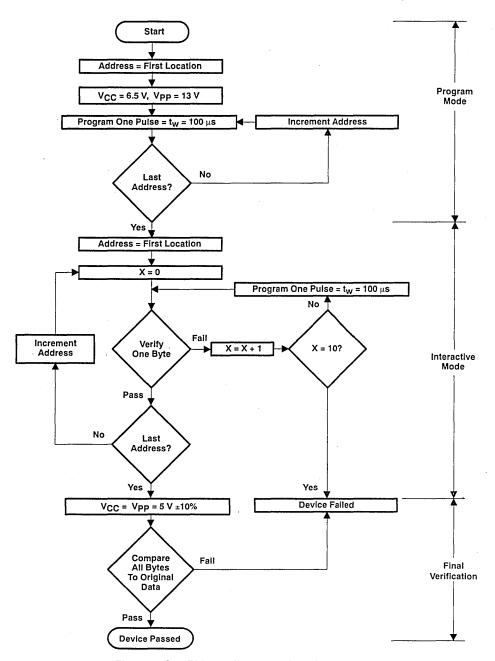
Figure 1. SNAP! Pulse Programming Flowchart
