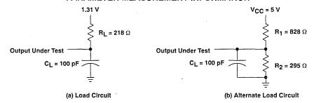
Figure 2. Load Circuits for Timing Parameters
