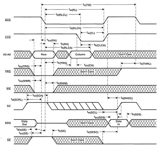
NOTES: 31. Random-mode Q outputs remain in the high-impedance state for the entire write-mode control.
