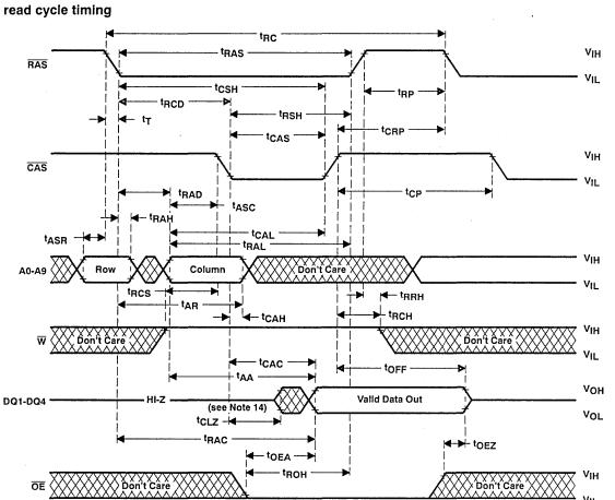
NOTE 14: Valid data is presented at the outputs after all access times are satisfied but may go from three-state to an invalid data state prior to the specified access times as the outputs are driven when CAS goes low.
