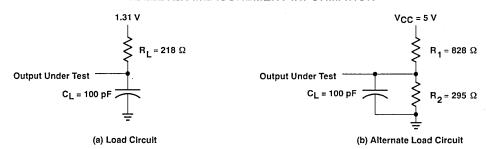
Figure 1. Load Circuits for Timing Parameters
