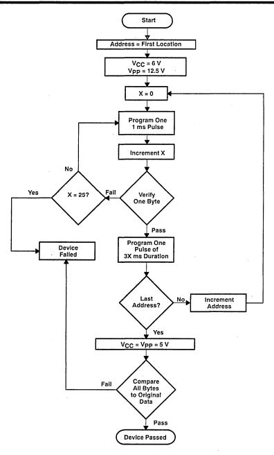
Figure 2. FAST Programming Flowchart
