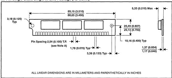
Note A: Each pin centerline is located within 0,25 (0.010) of its true longitudinal position.
