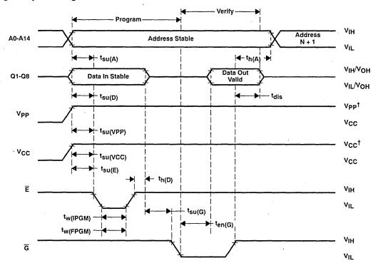
† 12.5-V Vpp and 6-V VCC for Fast programming, 13-V Vpp and 6.5-V VCC for SNAP! Pulse programming.
