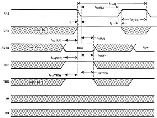
NOTE 30: In persistent write-per-bit function, W must be high during the refresh cycle.
