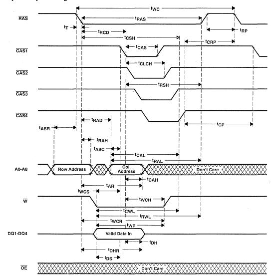
NOTES: 17. In order to hold the address latched by the first \$\overline{CASx}\$ going low, the parameter to must be met.
