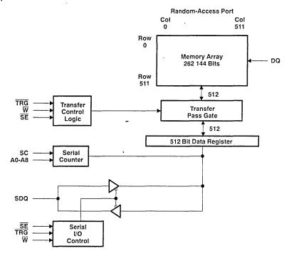
Figure 2. Block Diagram Showing One Random and One Serial I/O Interface
