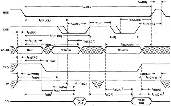
NOTE 25: A write cycle or a read-modify-write cycle can be mixed with the read cycles as long as the write and read-modify-write timing specifications are not violated.
