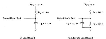
Figure 1. Load Circuits for Timing Parameters
