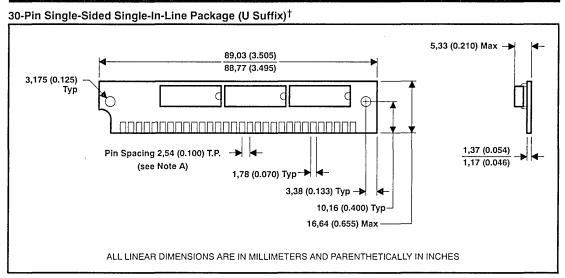
Note A: Each pin centerline is located within 0,25 (0.010) of its true longitudinal position.
