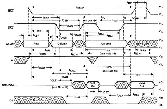
NOTES: 14. Valid data is presented at the outputs after all access times are satisfied but may go from three-state to an invalid data state prior to the specified access times as the outputs are driven when CAS goes low.
