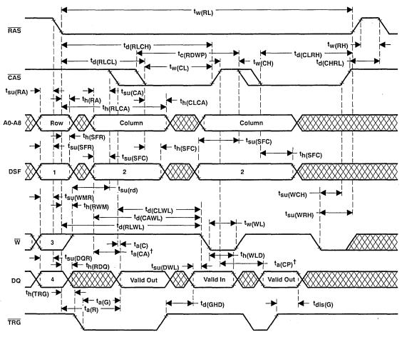
† Output may go from the high-impedance state to an invalid data state prior to the specified access time. NOTES: 25. See "Write Cycle State Table" for the logic state of "1", "2", "3", "4", and "5".
