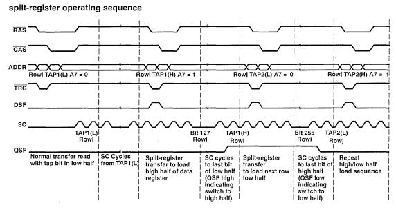
NOTES:36. In split register mode, data can be transferred from different rows to the low and high halves of the data register.
