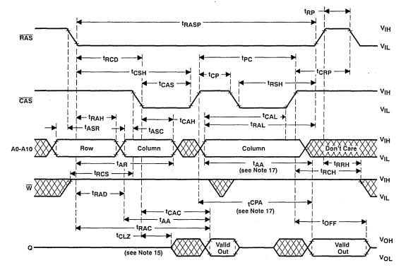
NOTES: 15. Valid data is presented at the output after all access times are satisfied. The output may go from three-state to an invalid data state prior to the specified access times as the output is driven when CAS goes low.
