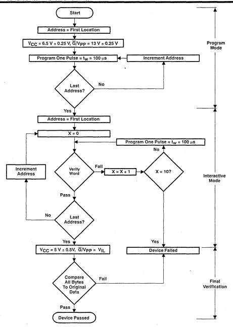
Figure 1. SNAP! Pulse Programming Flowchart
