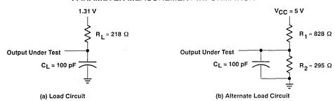
Figure 1. Load Circuits For Timing Parameters
