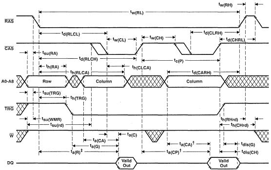
NOTE 28: A write cycle or a read-modify-write cycle can be mixed with the read cycles as long as the write and read-modify-write timing specifications are not violated.
