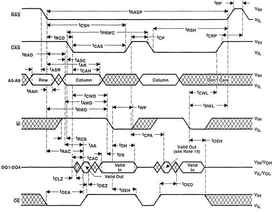
NOTES: 14. Valid data is presented at the outputs after all access times are satisfied but may go from three-state to an invalid data state prior to the specified access times as the outputs are driven when CAS goes low.
