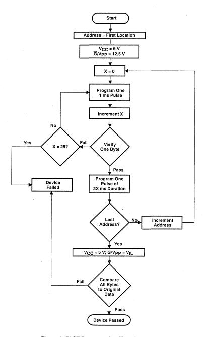
Figure 2. FAST Programming Flowchart
