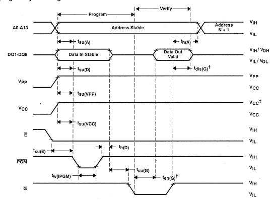
$<sup>^\</sup>dagger$   $t_{dis(G)}$  and  $t_{en(G)}$  are characteristics of the device but must be accommodated by the programmer. ‡ 13-V V<sub>PP</sub> and 6.5-V V<sub>CC</sub> for SNAP! Pulse programming.
