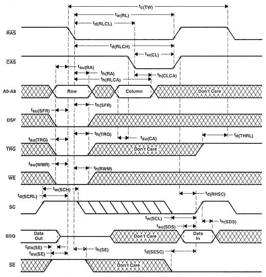
NOTES: 31. Random-mode Q outputs remain in the high-impedance state for the entire write-mode control.
