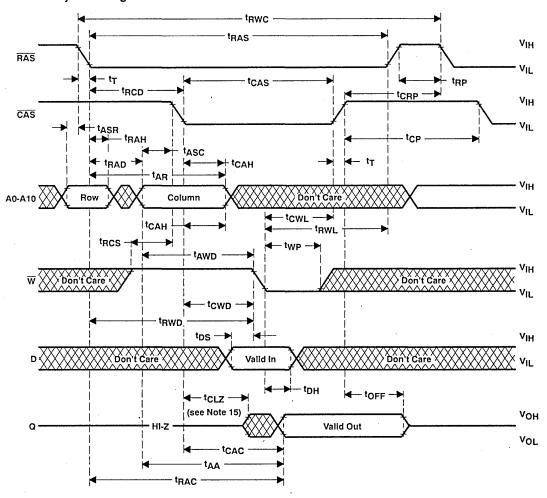
NOTE 15: Valid data is presented at the output after all access times are satisfied. The output may go from three-state to an invalid data state prior to the specified access times as the output is driven when CAS goes low.
