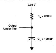
Figure 2. AC Testing Output Load Circuit
