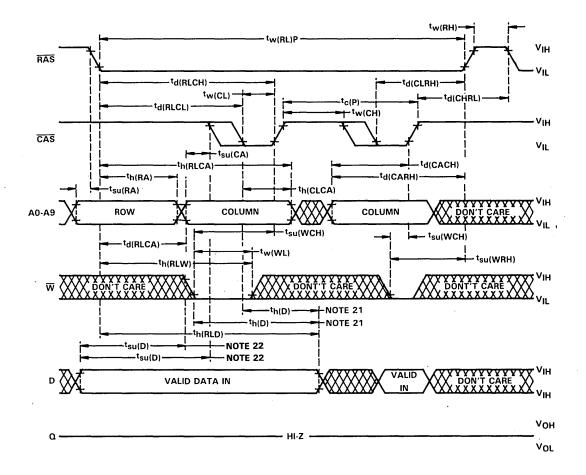
NOTES: 21. A read cycle or a read-modify-write cycle can be intermixed with write cycles as long as read and read-modify-write timing specifications are not violated.
