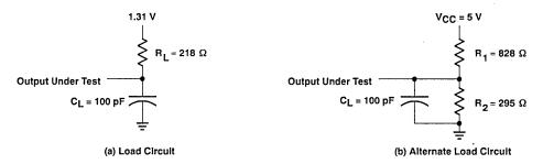
Figure 2. Load Circuits for Timing Parameters
