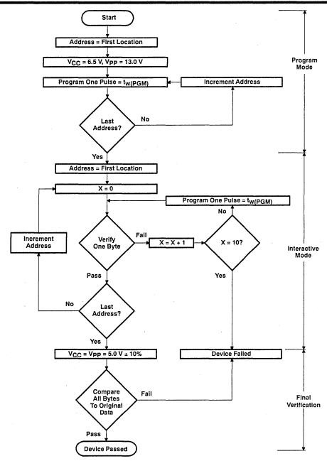
Figure 1. SNAP! Pulse Programming Flowchart
