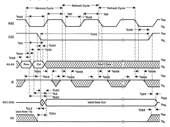
NOTE 14: Valid data is presented at the outputs after all access times are satisfied but may go from three-state to an invalid data state prior to the specified access times as the outputs are driven when CAS goes low.
