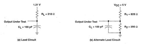
Figure 1. Load Circuits for Timing Parameters
