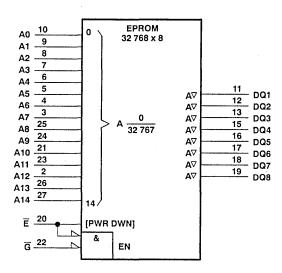
The address inputs are arranged in order of their assigned binary weights and the range of addresses are shown as  $A^{\frac{m}{n}}$  where m is the decimal equivalent of the lowest address and n is the highest. The outputs affected by these addresses are indicated by the letter A, as data inputs would also be if the device were a RAM.
