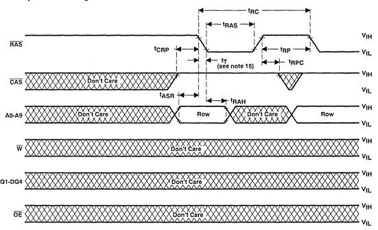
NOTE 15: Transition times (rise and fall) for  $\overline{RAS}$  and  $\overline{CAS}$  are to be a minimum of 3 ns and a maximum of 50 ns.
