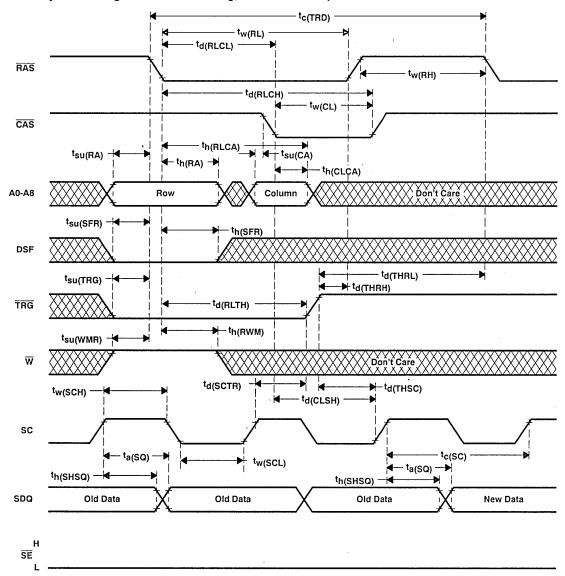
NOTES: 35. Random mode (Q outputs) remain in the high-impedance state for the entire memory to data register transfer cycle. The memory to data register transfer cycle is used to load the data registers in parallel from the memory array. The 512 locations in each data register are written into from the 512 corresponding columns of the selected row. The data that is transferred into the data registers may be either shifted out or transferred back into another row.
