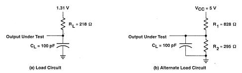
Figure 1. Load Circuits for Timing Parameters
