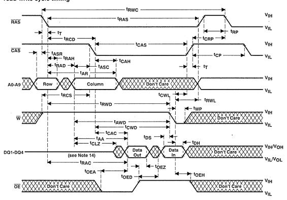
NOTE 14: Valid data is presented at the outputs after all access times are satisfied but may go from three-state to an invalid data state prior to the specified access times as the outputs are driven when OAS goes low.
