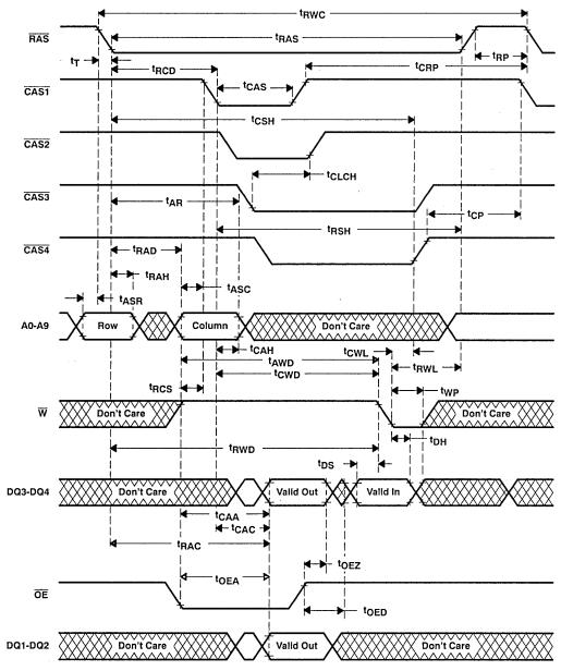
NOTES: 17. In order to hold the address latched by the first CASx going low, the parameter t<sub>CLCH</sub> must be met.
