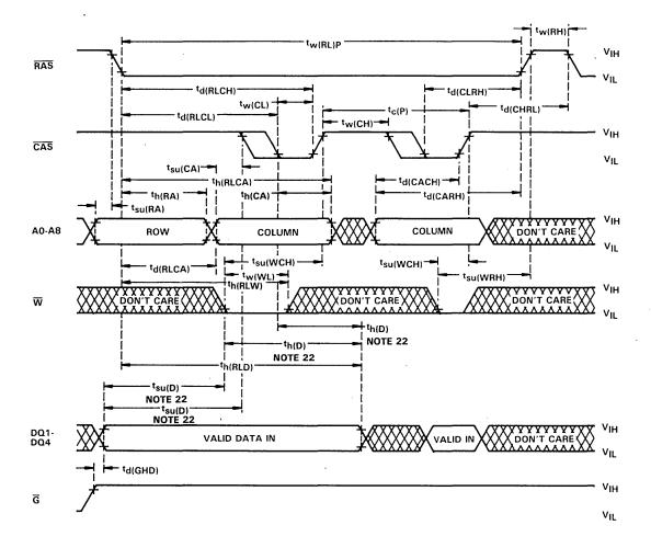
NOTES: 21. A read cycle or a read-modify-write cycle can be intermixed with the write cycles as long as the read and read-modify-write timing specifications are not violated.
