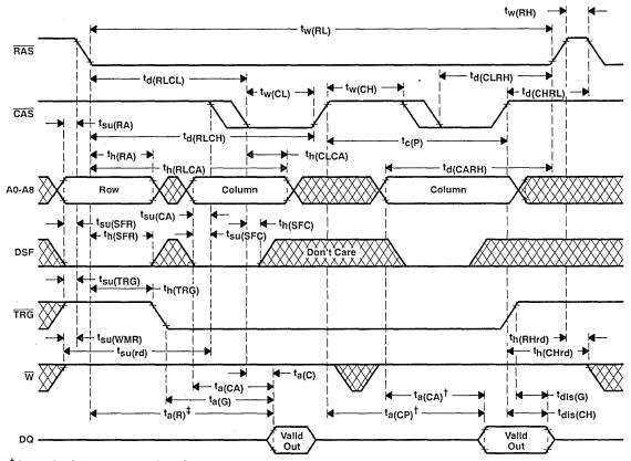
$<sup>^\</sup>dagger$  Access time is  $t_{a(CP)}$  or  $t_{a(CA)}$  dependent.  $^\ddagger$  Output may go from high-impedance state to an invalid data state prior to the specified access time.
