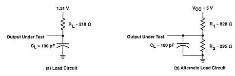
Figure 2. Load Circuits for Timing Parameters
