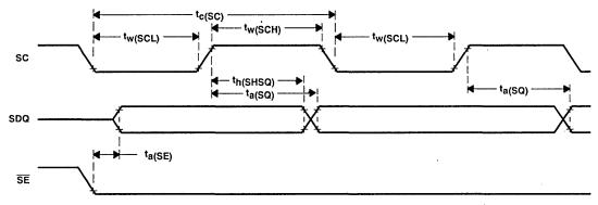
NOTE: 10. When the odd tap is used (tap addresses can be 0-511, and odd taps are 1,3,5 ... etc.), the cycle time for SC in the first serial data out cycle needs to be 40 ns minimum.
