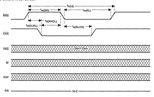
NOTE 30: In persistent write-per-bit function,  $\overline{W}$  must be high during the refresh cycle.
