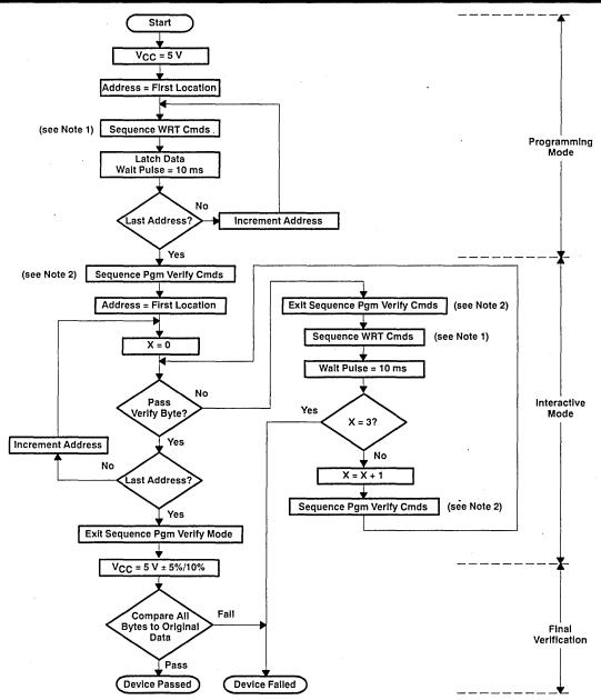
NOTES: 1. Upon the three-step sequence completion, the device is latched into the programming mode. The byte is latched and the byte programming operation starts if a subsequent rising edge of W is not detected within 100 μs.
