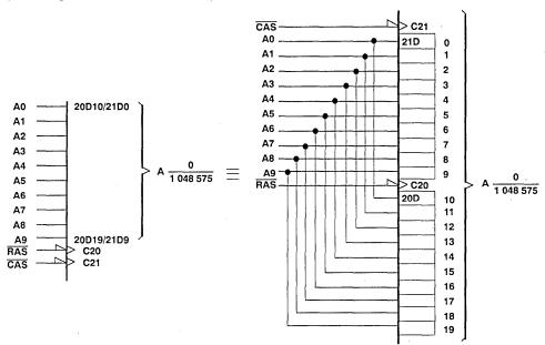
When  $\overline{RAS}$  goes low, it momentarily enables (through C20,  $\triangleright$  indicates a dynamic input) the D inputs of the ten address registers 10 through 19. When  $\overline{CAS}$  goes low, it momentarily enables (through C21) the D inputs of the ten address registers 0 through 9. The outputs of the address registers are in 20 internal address lines that select 1 of 1 048 576 cells.
