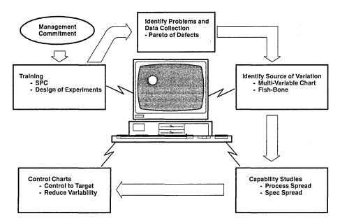
Figure 3. Computer-Aided Statistical Process Control
