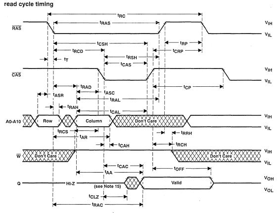
NOTE 15: Valid data is presented at the output after all access times are satisfied. The output may go from three-state to an invalid data state prior to the specified access times as the output is driven when CAS goes low.
