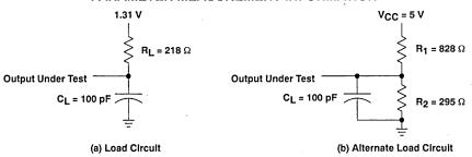
Figure 1. Load Circuits for Timing Parameters
