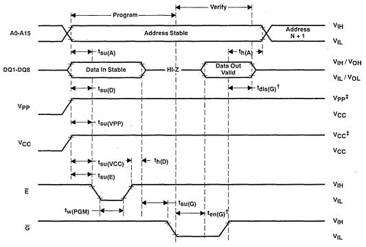
$<sup>^\</sup>dagger$  t<sub>dis(G)</sub> and t<sub>en(G)</sub> are characteristics of the device but must be accommodated by the programmer.  $^\ddagger$  13.0-V Vpp and 6.5-V V<sub>CC</sub> for SNAP! Pulse programming.
