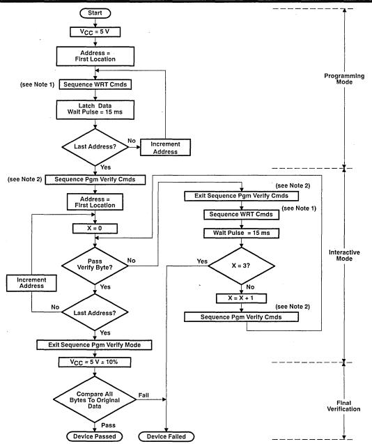
NOTES: 1. Upon the three-step sequence completion, the device is latched into programming mode. The byte is latched and the byte programming operation starts if a subsequent rising edge of W is not detected within 100 μs.
