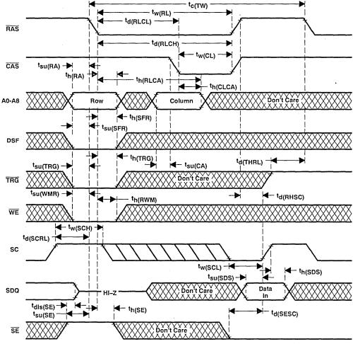
NOTES:31. Random-mode Q outputs remain in the high-impedance state for the entire write-mode control. 32. SE must be high as RAS falls in order to perform a write-mode control cycle.
