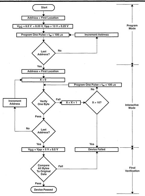
Figure 1. SNAP! Pulse Programming Flowchart
