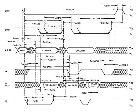
NOTES: 18. Output may go from high impedance to an invalid data state prior to the specified access time.
