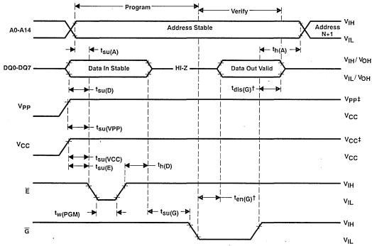
$<sup>^{\</sup>dagger}$  t<sub>dis(G)</sub> and t<sub>en(G)</sub> are characteristics of the device but must be accommodated by the programmer.  $^{\ddagger}$  13-V V<sub>PP</sub> and 6.5-V V<sub>CC</sub> for SNAP! Pulse programming.
