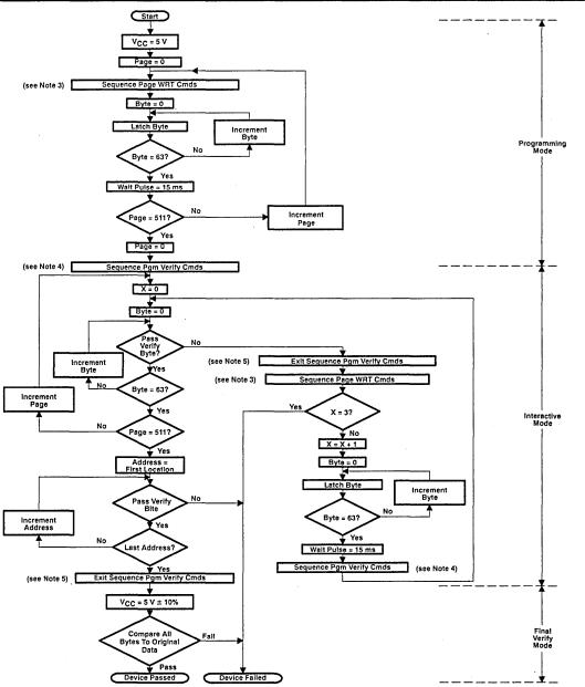
NOTES: 3. Upon the three-step sequence completion, the device is latched into programming mode. From 2 up to 64 bytes are latched at a rate of 1 µs up to 100 µs per byte.
