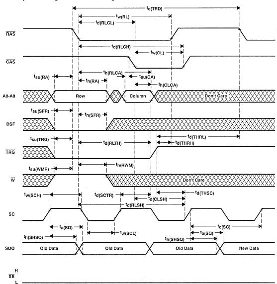
NOTES: 38. Random mode (Q outputs) remain in the high-impedance state for the entire memory to data register transfer cycle. The memory to data register transfer cycle is used to load the data registers in parallel from the memory array. The 512 locations in each data register are written into from the 512 corresponding columns of the selected row. The data that is transferred into the data registers may be either shifted out or transferred back into another row.
