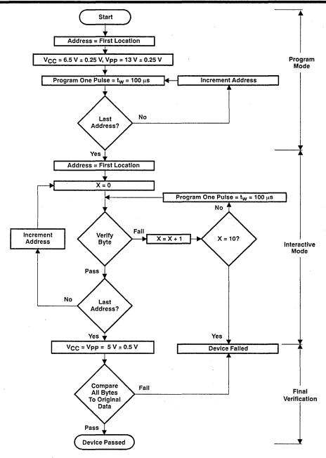
Figure 1. SNAP! Pulse Programming Flowchart
