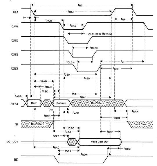
NOTES: 17. In order to hold the address latched by the first  $\overline{\text{CASx}}$  going low, the parameter t<sub>CLCH</sub> must be met.
