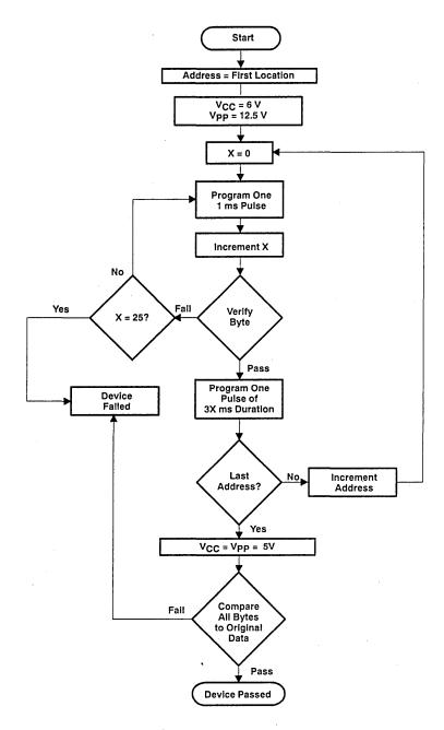
Figure 2. FAST Programming Flowchart
