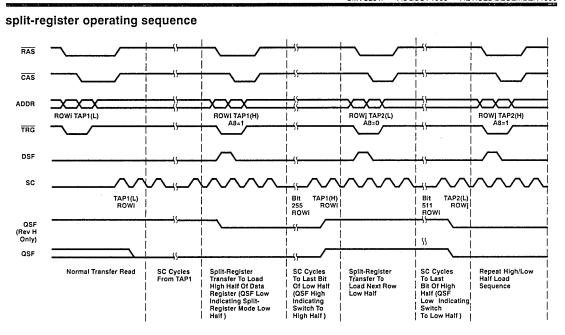
NOTES: 38. In the split-register mode, data can be transferred from different rows to the low and high halves of the data register.
