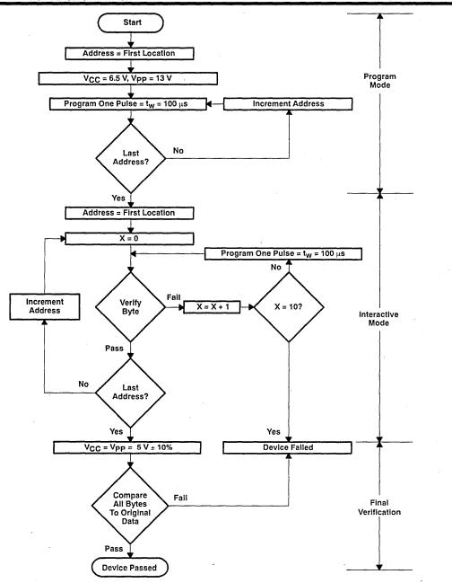
Figure 1. SNAP! Pulse Programming Flowchart
