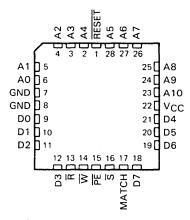
MATCH output. A low-level output on  $\overline{PE}$  signifies a parity error in the internal RAM data.  $\overline{PE}$  is an N-channel open-drain output for easy OR-tying. During a write cycle ( $\overline{S}$  and  $\overline{W}$  low), data on D0-D7 plus generated odd parity are written in the 9-bit memory location addressed by A0-A10. Also during write, a parity error may be forced by holding  $\overline{PE}$  low.
