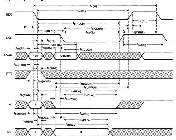
NOTE 26: See "Write Cycle State Table" for the logic state of "1", "2", and "3".
