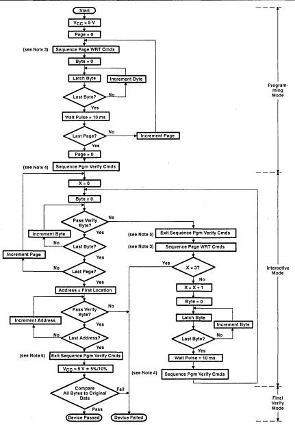
NOTES: 3. Upon the three-step sequence completion, the device is latched into the programming mode. From 2 up to 32 bytes are latched at a rate of 1 µs up to 100 µs per byte. There are 1024 pages.
