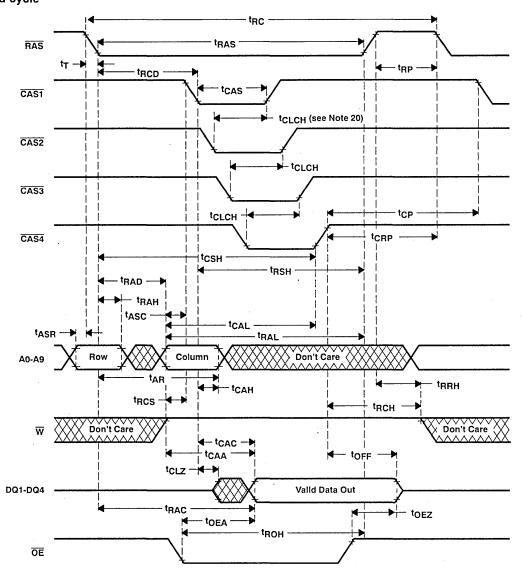
NOTES:17. In order to hold the address latched by the first  $\overline{\text{CASx}}$  going low, the parameter t<sub>CLCH</sub> must be met.
