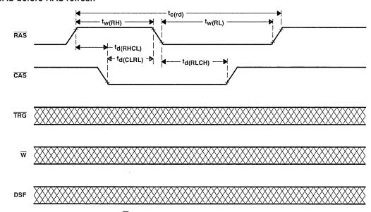
NOTE 29: In persistent write-per-bit function,  $\overline{W}$  must be high during the refresh cycles.
