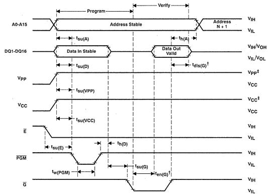
$^\dagger$   $t_{dis(G)}$  and  $t_{en(G)}$  are characteristics of the device but must be accomodated by the programmer.  $^\ddagger$  13-V Vpp and 6.5-V VCC for SNAP! Pulse programming.
