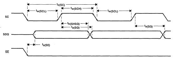
NOTES: 8. For mid-line load, t<sub>C</sub>(SC) = 50 ns for Revision I and subsequent revisions; t<sub>C</sub>(SC) = 55 ns for Revision H only. For split-register, t<sub>C</sub>(SC) = 40 ns for Revision H only.
