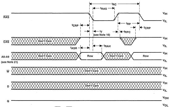
NOTES: 16. Transition times (rise and fall) for  $\overline{RAS}$  and  $\overline{CAS}$  are to be minimum of 3 ns and maximum of 50 ns. 21. A10 is a don't care.
