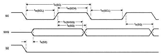
NOTE 10: When the odd tap is used (tap addresses can be 0-511, and odd taps are 1,3,5 ... etc.), the cycle time for SC in the first serial data out cycle needs to be 70 ns minimum.
