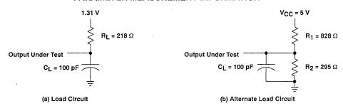
Figure 1. Load Circuits for Timing Parameters
