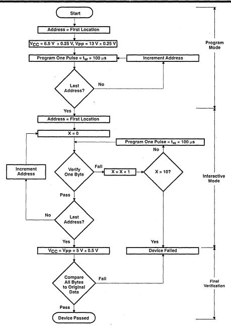
Figure 1. SNAP! Pulse Programming Flowchart
