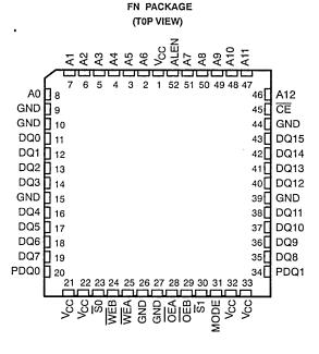
circuits. The 'ACT2140A was designed so that it will interface directly with the Intel 82385 cache controller. Significant reductions in memory component count, board area, and power dissipation can be achieved by using this device. When using the 2-way mode, two 'ACT2140As replace 16 4K x 4 static RAMs, two latches, eight bidirectional transceivers, and one AND gate.
