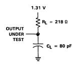
(b) ALTERNATE LOAD CIRCUIT
