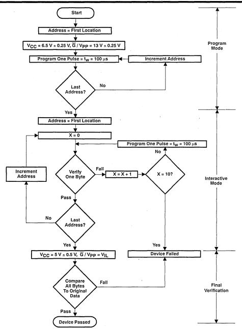
Figure 1. SNAP! Pulse Programming Flowchart
