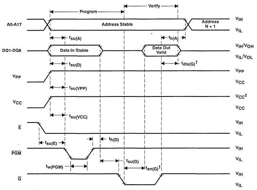
$<sup>^{\</sup>dagger}$   $t_{dis(G)}$  and  $t_{en(G)}$  are characteristics of the device but must be accommodated by the programmer.
