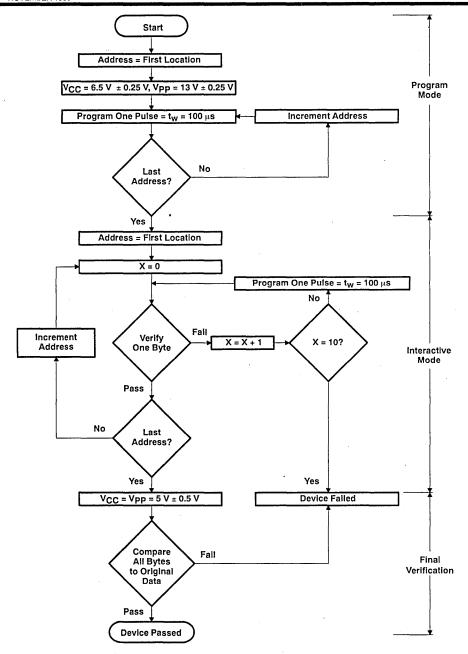
Figure 1. SNAP! Pulse Programming Flowchart
