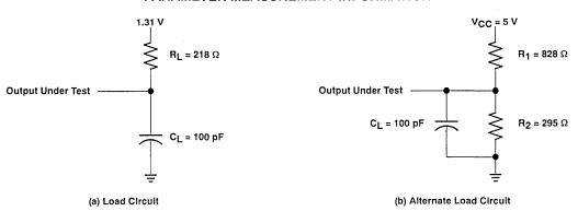
Figure 1. Load Circuits for Timing Parameters
