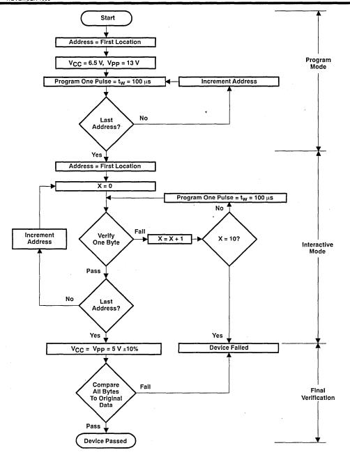
Figure 1. SNAP! Pulse Programming Flowchart
