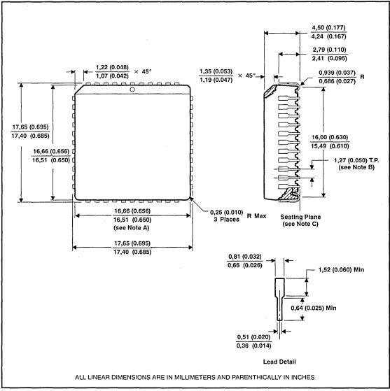
NOTES: A. Centerline of center pin each side is within 0,10 (0.004) of package centerline as determined by this dimension.
