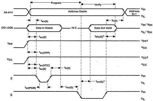
$<sup>^\</sup>dagger$  t<sub>dis(G)</sub> and t<sub>en(G)</sub> are characteristics of the device but must be accomodated by the programmer.  $^\ddagger$  13-V V<sub>PP</sub> and 6.5-V V<sub>CC</sub> for SNAP! Pulse programming.
