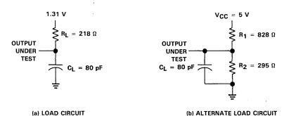
FIGURE 1. LOAD CIRCUITS FOR TIMING PARAMETERS
