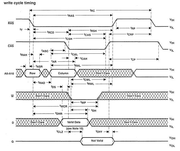
NOTE 15: Valid data is presented at the output after all access times are satisfied. The output may go from three-state to an invalid data state prior to the specified access times as the output is driven when CAS goes low.
