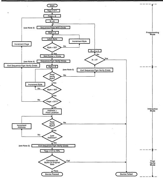
NOTES: 3. Upon the three-step sequence completion, the device is latched into programming mode. From 2 up to 64 bytes are latched at a rate of 1  $\mu$ s up to 100  $\mu$ s per byte.
