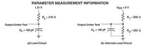
Figure 1. Load Circuits For Timing Parameters
