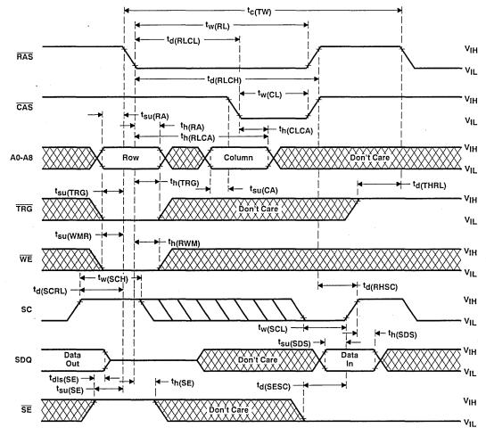
NOTES: 28. Random-mode Q outputs remain in the high-impedance state for the entire write-mode control.
