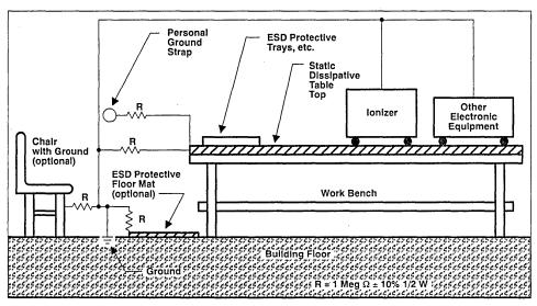
All electrical equipment sitting on the conductive table top must be hard grounded but must be isolated from the static disspative work surface. NOTE: Earth ground is not computer ground or RF ground or any other limited-type ground.
